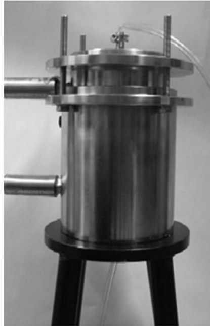
Figure 2-5 Experimental mold for measurement of out-of-plane permeability (Song et al., 2009)
