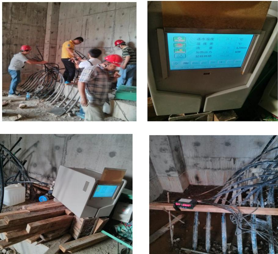
**Figure 6.4** The on-site photos of heat transfer experiments of energy piles
