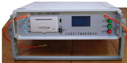
**Figure 6.2 The photo of thermophysical tester**
