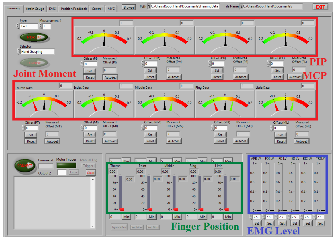
Figure 3.7. Graphical User Interface (GUI) of the hand exoskeleton robot system program. Highlighted in red is the display for each joint moment. On the top, from left to right, are the PIP joint moments of the index, middle, ring, and little finger; on the bottom, from left to right, are the MCP joint moments of the thumb, index, middle, ring, and little finger. The 5 finger positions are shown in the bars highlighted in green; and the EMG level display for 6 muscles of interests, namely APB, FDI, FD, ED, BIC, and TRI, are highlighted in blue.
