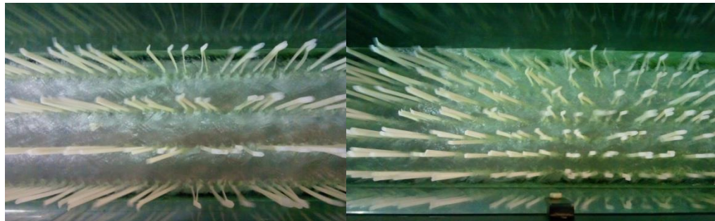
Plate 5.1: Snapshots of flow through simulated vegetation with constant S_x
