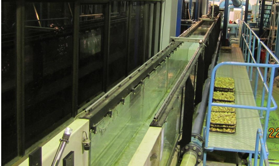
Plate 4.1: Tilting, slope – adjustable rectangular flume
