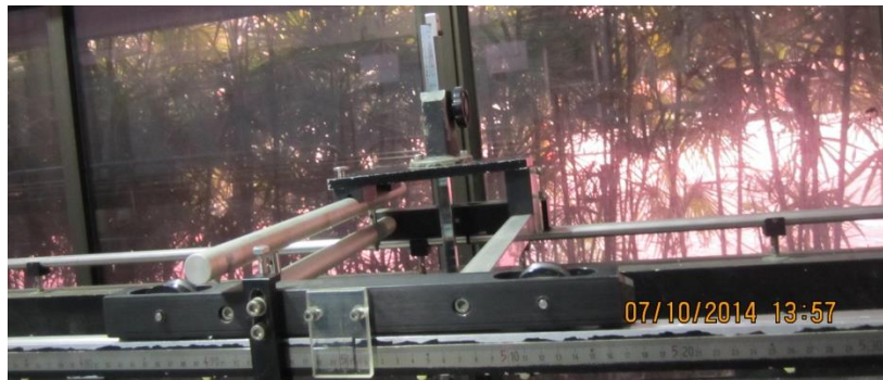
Plate 4.2: Movable wheeled trolleys with Vernier point gauge
