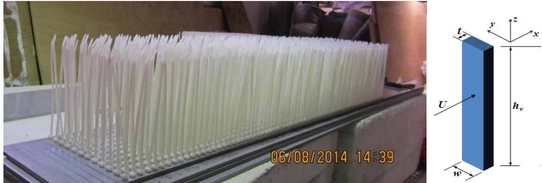
Plate 4.7: Modelled vegetation elements and geometrical characteristics
