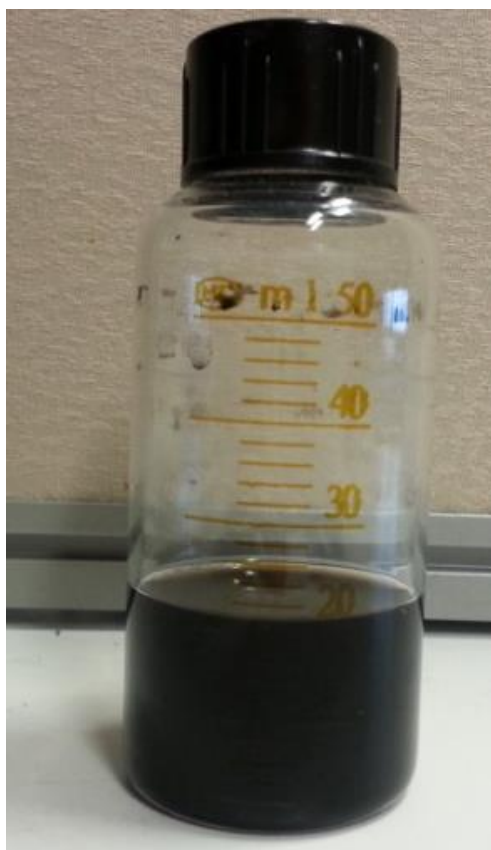
Figure 3.18. The DI water- SWCNT solution after 6 hours sonication.
