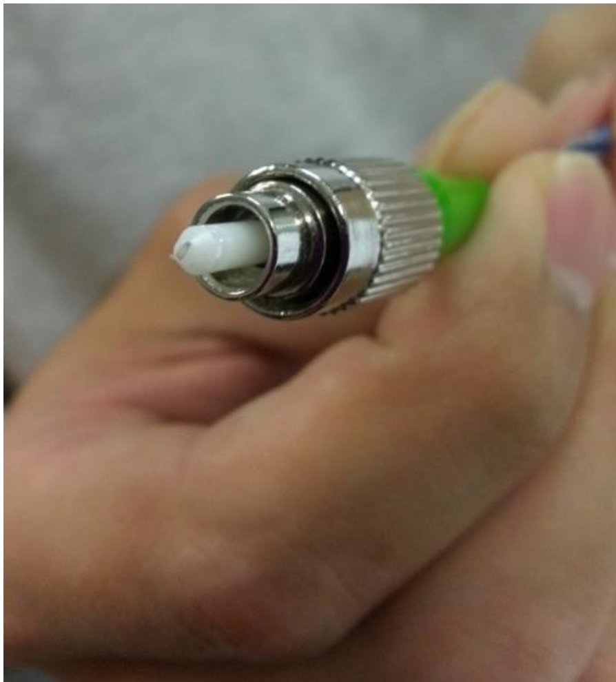
Figure 3.31. And the SWCNT-PVA film coated on the connector end
