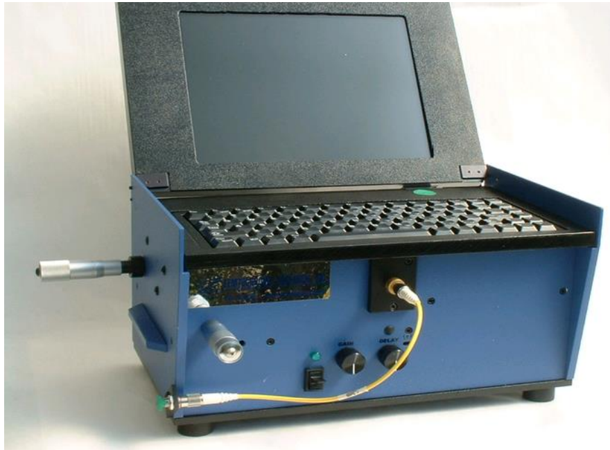
Figure 3.17 Femtochrome FR-103XL Autocorrelator.
