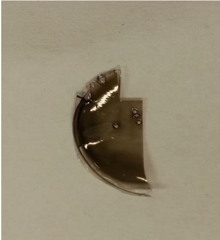
Fig. 3.32: The SWCNT-PVA thin film.
