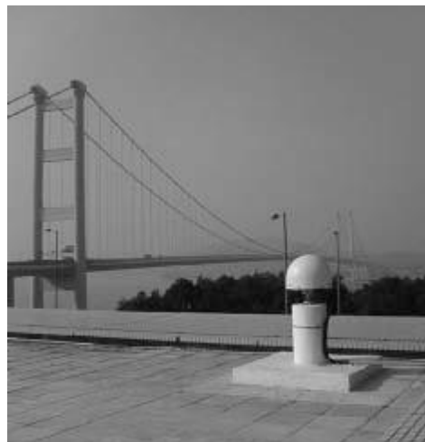
Figure 4.5 A GPS reference station on the roof of a storage building
