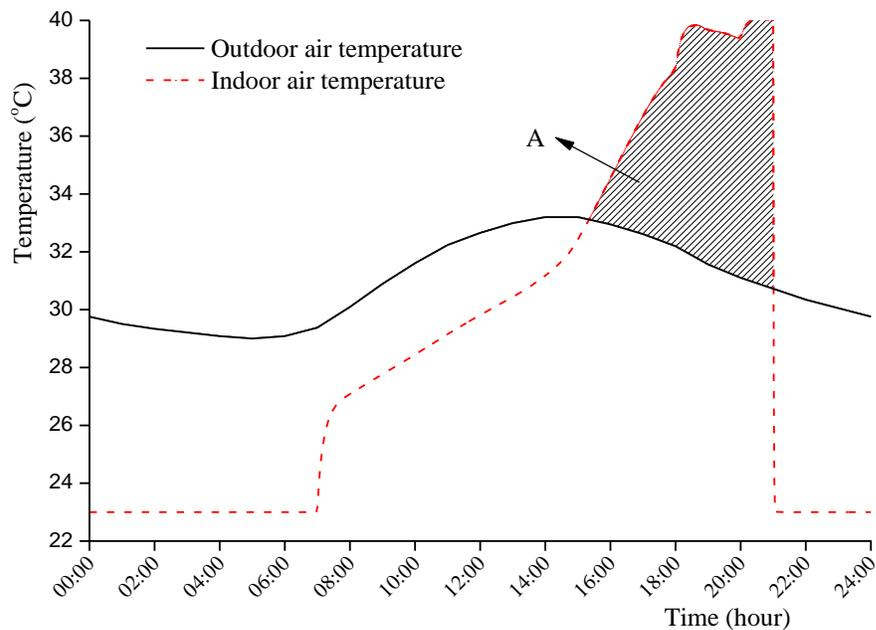
Figure 6.4 Simulated variation profile of hourly indoor air temperature in the west-facing bedroom in the summer design day
