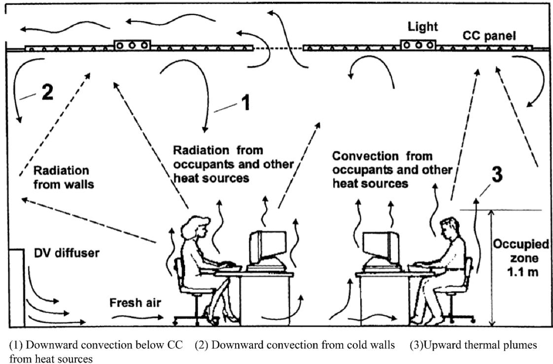
Figure 2.9 The convective and radiative heat transfer inside a room with a ceiling radiant cooling panel system (Novoselac and Srebric 2002)
