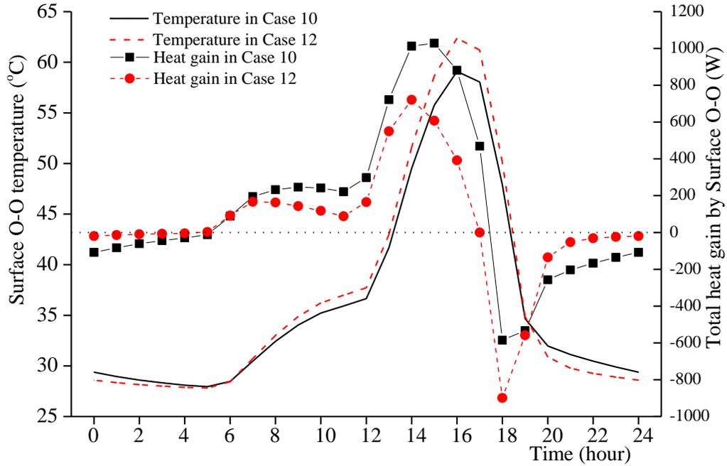
Figure 6.16 The simulated surface temperatures and the total heat gains on Surface O-O in Case 10 and Case 12
