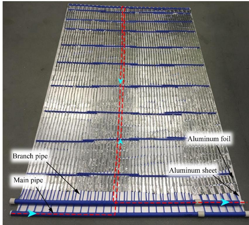
(a) The inner construction of the radiant panel
