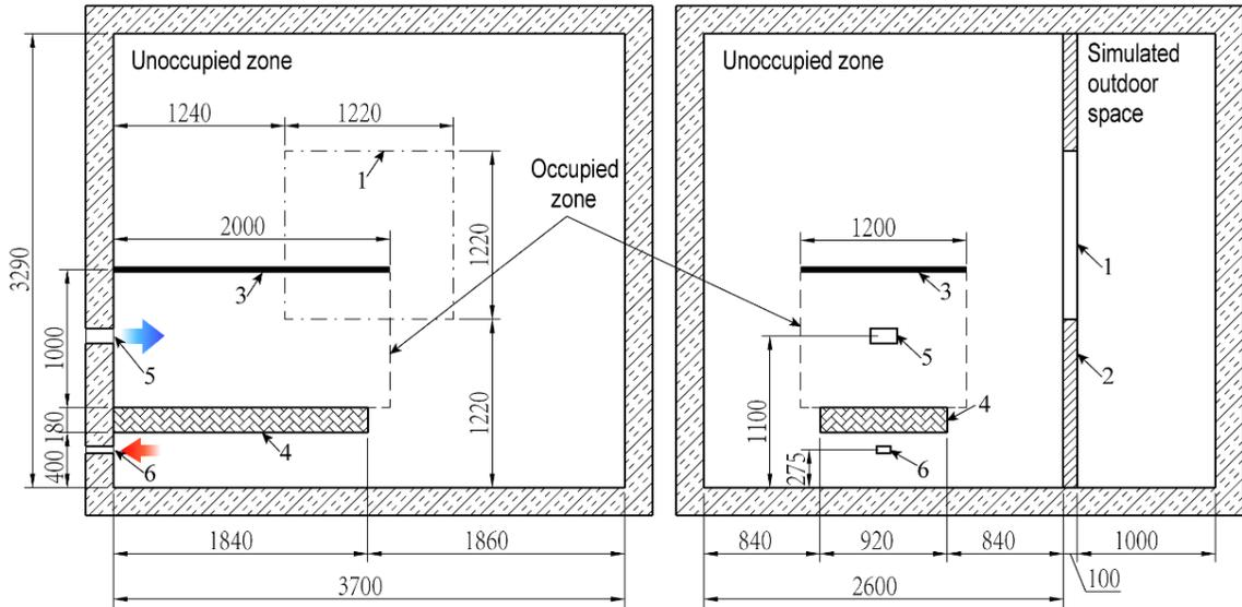
1. Simulated external window 2. Simulated external wall 3. Radiant panel 4. Mattress bed
