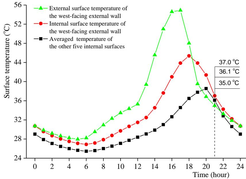
Figure 6.5 Simulated variation profiles for hourly surface temperatures in the west-facing bedroom in the summer design day
