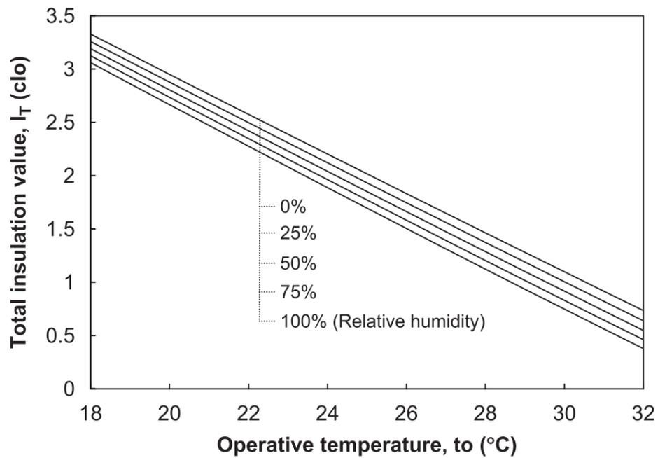
Figure 2.3 Relationships between operative temperature and the total insulation value ( $v \leq 0.15$  m/s) (Lin and Deng 2008a)
