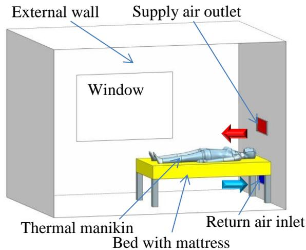
Figure 2.8 The improved bed-based TAC systems (Mao et al. 2013)
