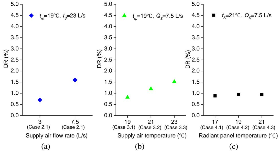
Figure 4.13 Averaged DR values in Group 2, 3 and 4 experiments in the occupied zone when using the R-TAC system
