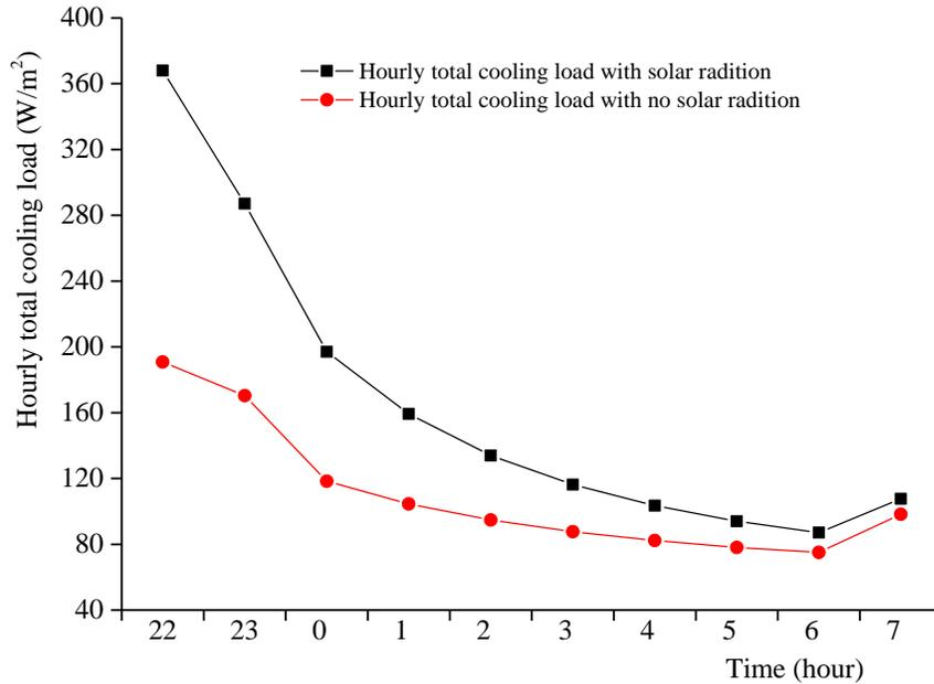
Figure 6.6 The comparison between the total cooling load at nighttime under the condition with solar radiation and that with no solar radiation in the simulated bedroom in the summer design day
