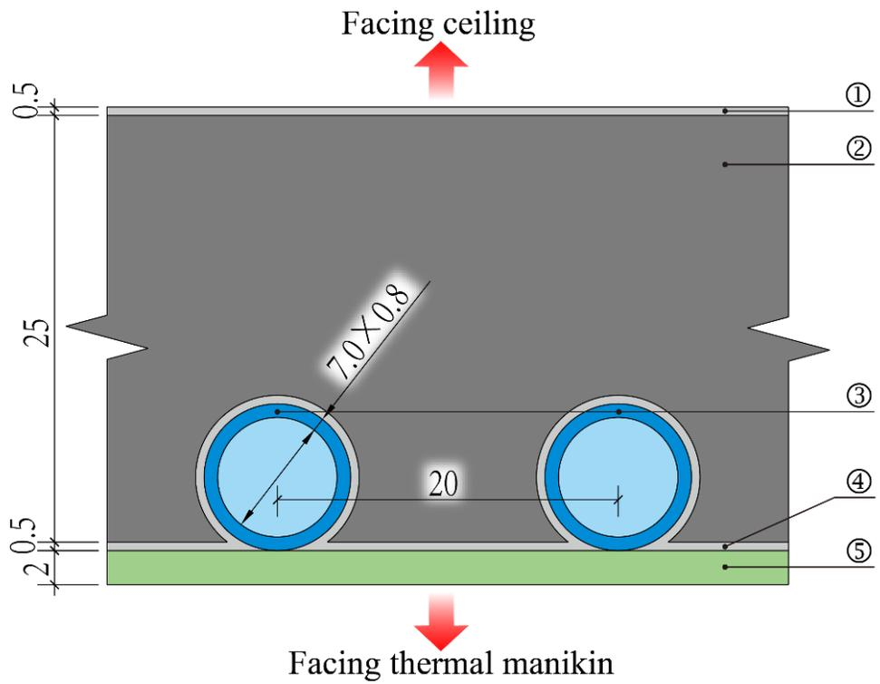
①④ Aluminum foil ② Thermal insulation layer ③ Water pipes ⑤ Aluminum sheet
