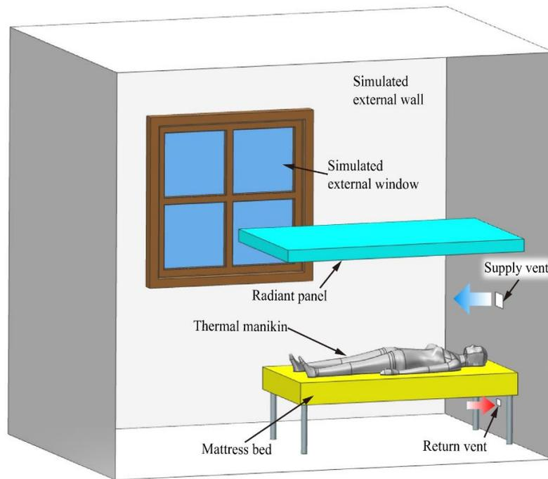
Figure 4.4 A 3-D view of the experimental bedroom and the prototype R-TAC system
