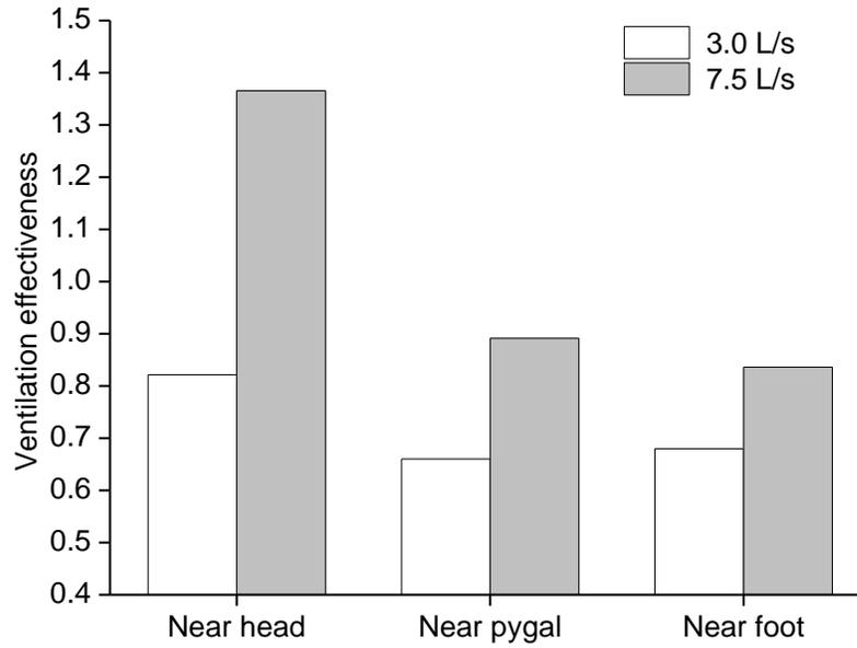
Figure 4.12 Measured ventilation effectiveness at three regions near three different body parts of the manikin at two different fresh air flow rates
