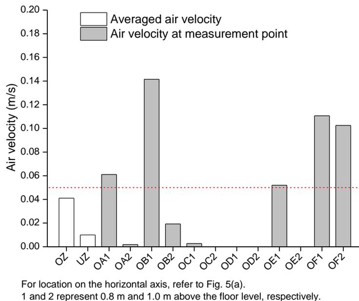
Figure 4.9 Averaged air velocities in the two zones and air velocity distribution in the occupied zone for experimental Case 1.1
