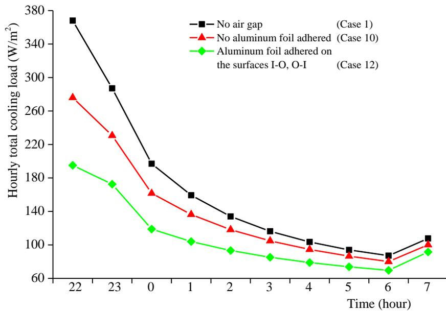
Figure 6.15 The simulated hourly total cooling loads in the bedroom in Case 1, 10 and 12 in the summer design day
