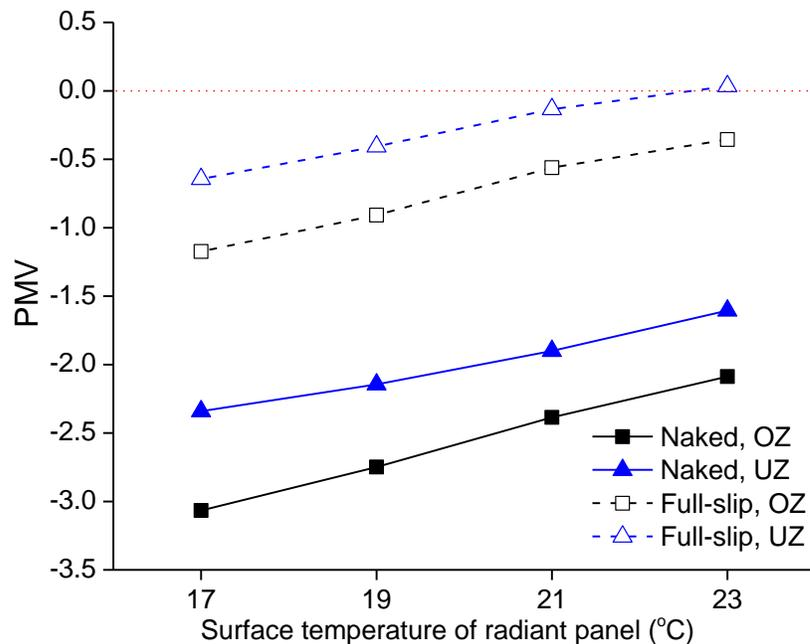
Figure 4.10 The evaluated PMV values based Group 1 experimental results in the occupied/unoccupied zones with two bedding insulations at different surfaces temperatures of the radiant panel
