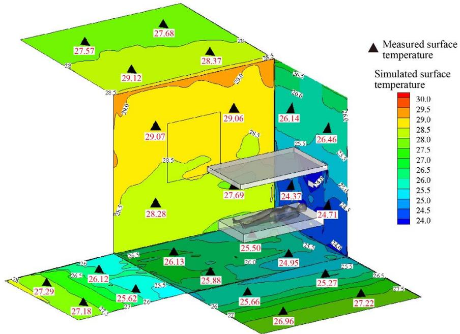
Figure 5.4 Comparison between the measured and simulated surface temperatures of six bedroom envelopes
