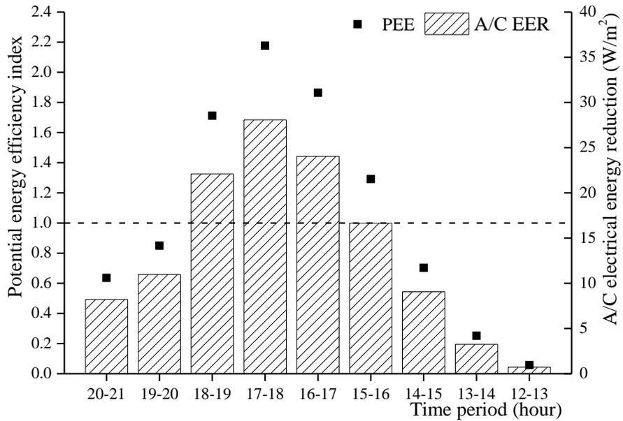
Figure 6.14 The simulation results of ventilating the air gap for only one hour during unoccupied period between 12:00 and 21:00 in Case 11
