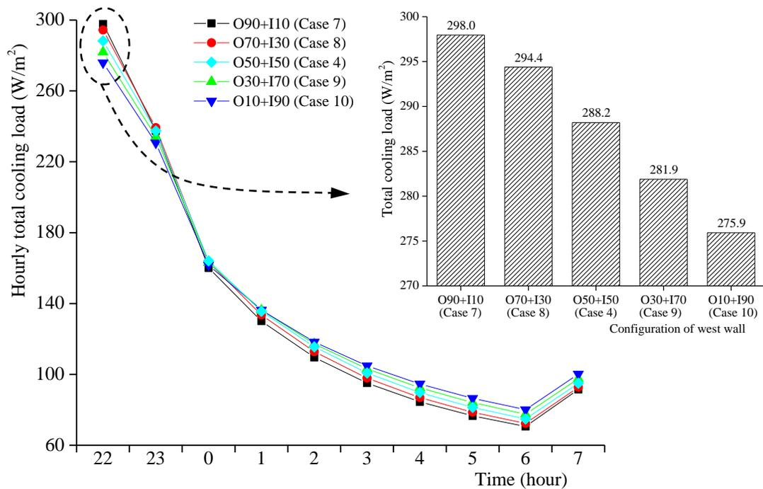
Figure 6.11 The total nighttime cooling load in the bedroom with varying width of inside and outside concrete layers of the west-facing external wall in the studied bedroom in the summer design day
