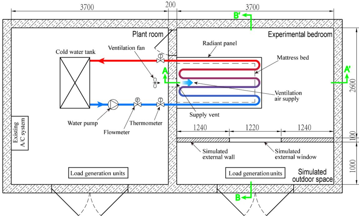
Figure 4.1 The schematics of the complete experimental setup for a prototype R-TAC system (unit: mm)
