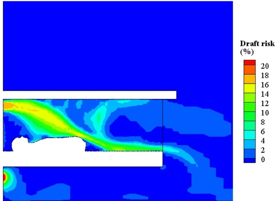
Figure 5.13 DR field in the bedroom when using the R-TAC system for Case L1.1
