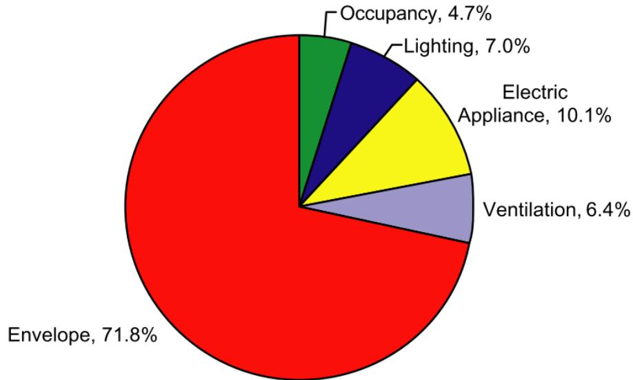
Figure 2.6 Percentage breakdown of the total cooling load for the west-facing bedroom at the A/C starting time (Lin and Deng 2004)
