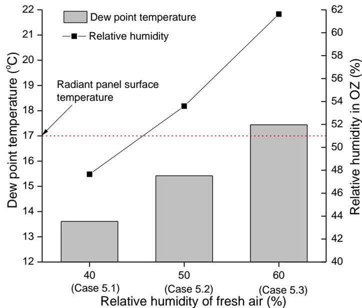
Figure 4.15 Averaged dew point temperature and relative humidity in the occupied zone for Group 5 experiments at different relative humidities of fresh air
