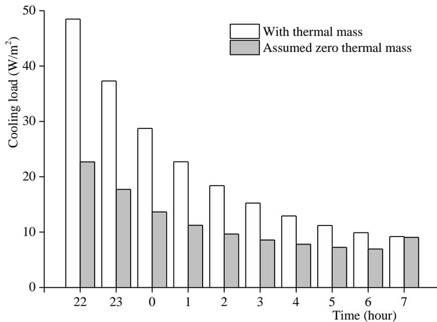
Figure 6.7 The simulated hourly nighttime cooling load due to the west-facing external wall with thermal mass and that without thermal mass
