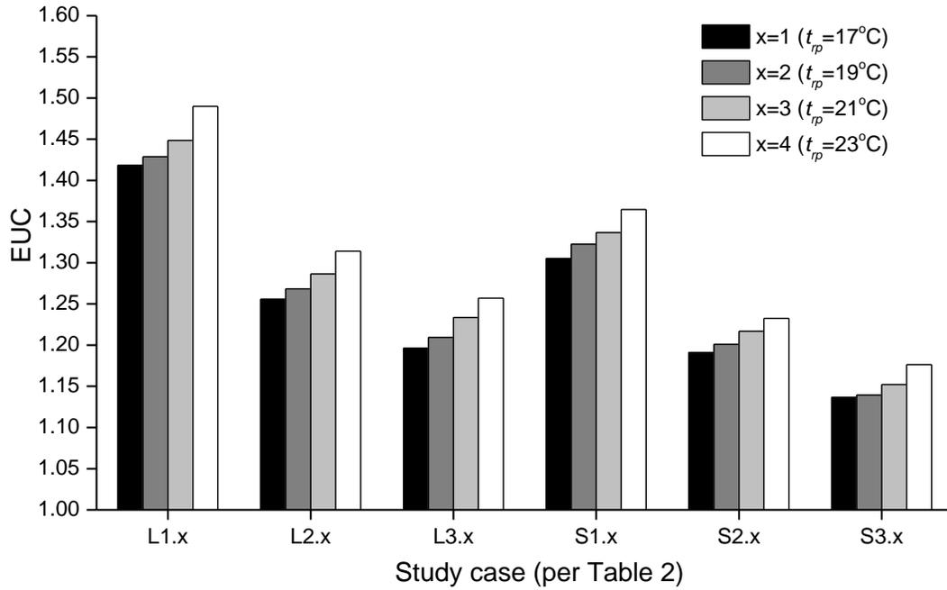
Figure 5.8 EUC values in the experimental bedroom when using R-TAC system at different study cases
