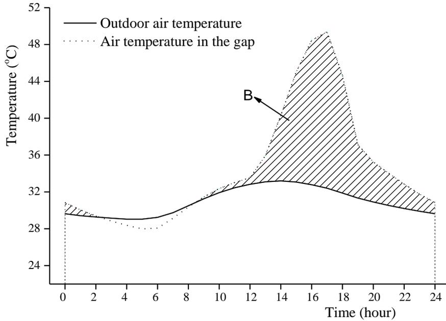
Figure 6.12 The simulated profiles of the air temperature in the air gap and outdoor air temperature in the summer design day in Case 10
