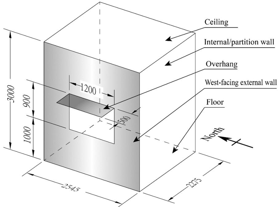
Figure 6.2 The details of the simulated bedroom (B3 in Apartment 6\_W)
