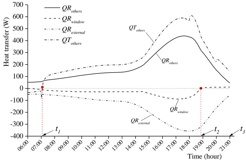
Figure 6.8 Simulated radiative heat exchanges within the bedroom at daytime in the summer design day
