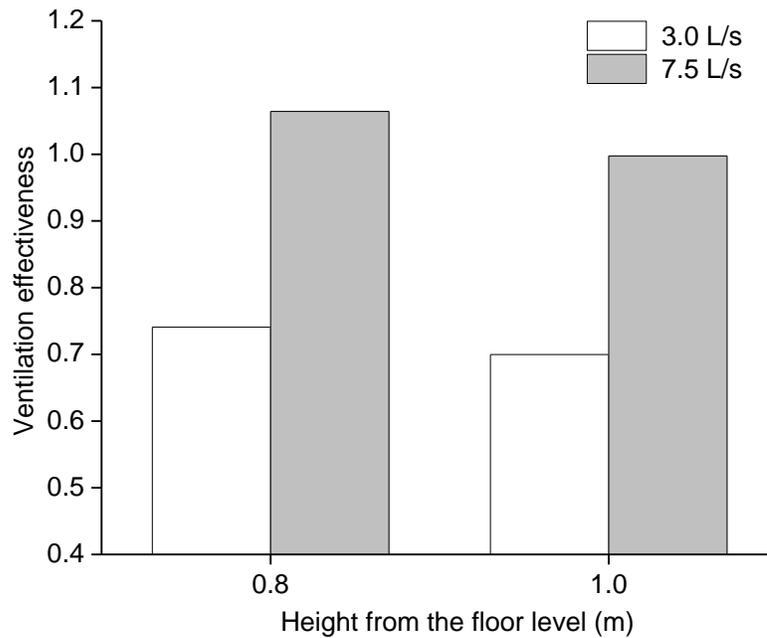
Figure 4.11 Measured ventilation effectiveness based on Group 2 experimental results at two different heights at two different fresh air flow rates
