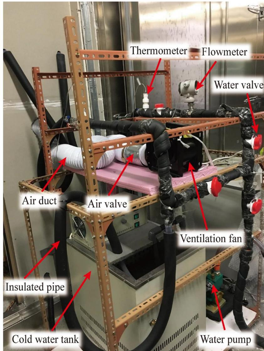
Photo 3 Water cooling system and ventilation system in the plant room
