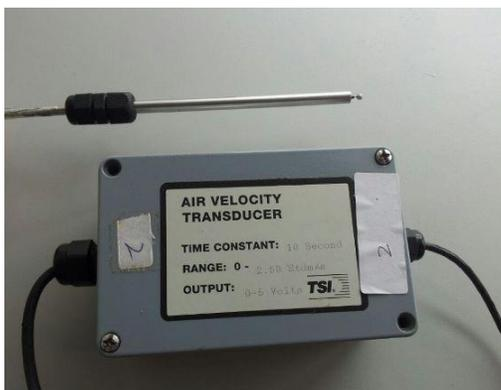
Photo 9 Air velocity transducer
