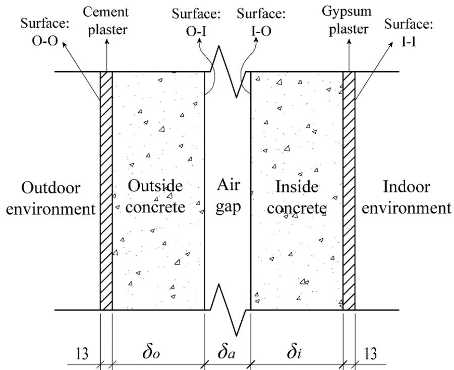
Figure 6.9 Configuration of the west-facing external wall in the simulated bedroom
