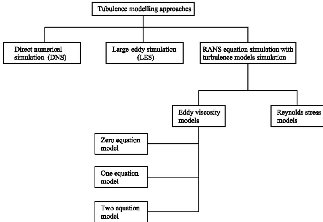
Figure 2.10 The classification of different turbulence modeling methods (Zhai et al. 2007)
