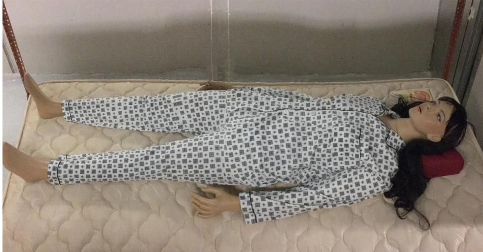
Figure 4.6 The thermal manikin used in the experiments
