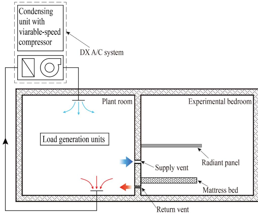
Figure 4.2 The existing DX A/C system in the plant room
