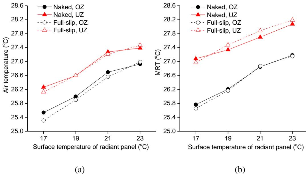
Figure 4.8 Indoor air temperatures and MRTs in Group 1 experimental cases
