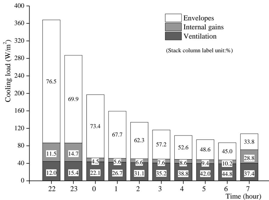
Figure 6.3 The simulated total hourly cooling loads at nighttime and their percentage breakdowns for the studied bedroom in the summer design day
