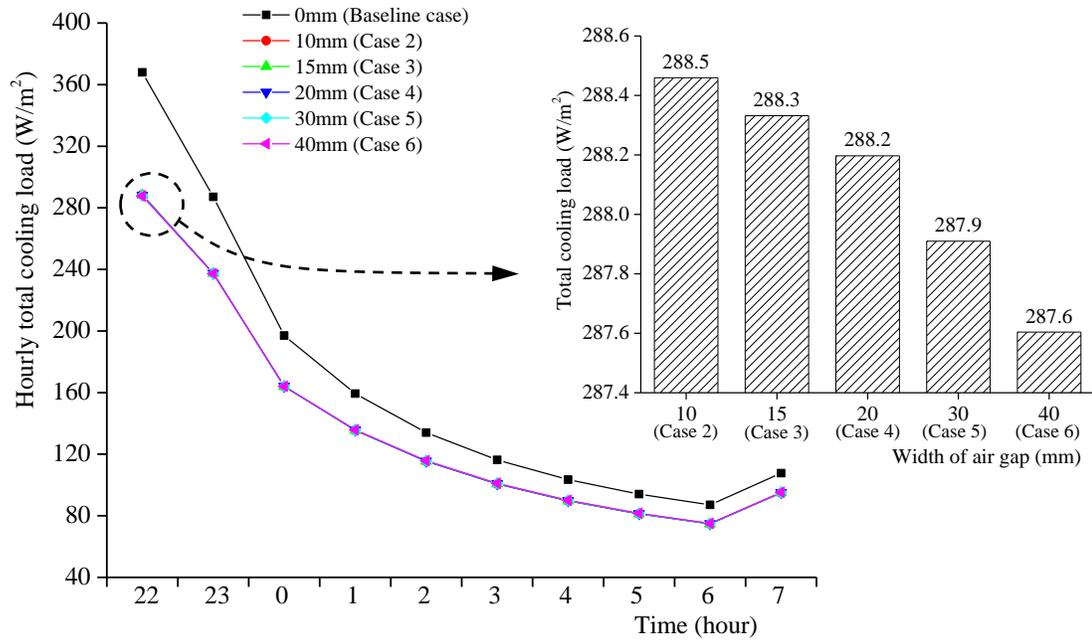
Figure 6.10 The simulated total nighttime cooling load in the bedroom with different widths of air gaps in the external wall
