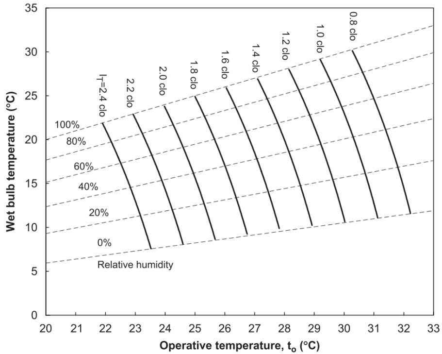
Figure 2.2 Comfort lines at different total insulation values ( $v \leq 0.15$  m/s) (Lin and Deng 2008a)
