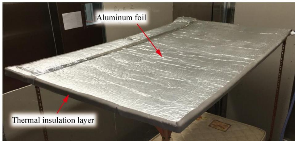
(b) The surface of the radiant panel facing ceiling
