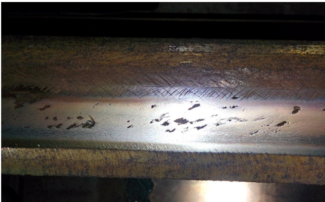
Figure 4. Significant roughness on railtrack, taken on-site measurement (July 2015, nearby Quarry Bay station).
