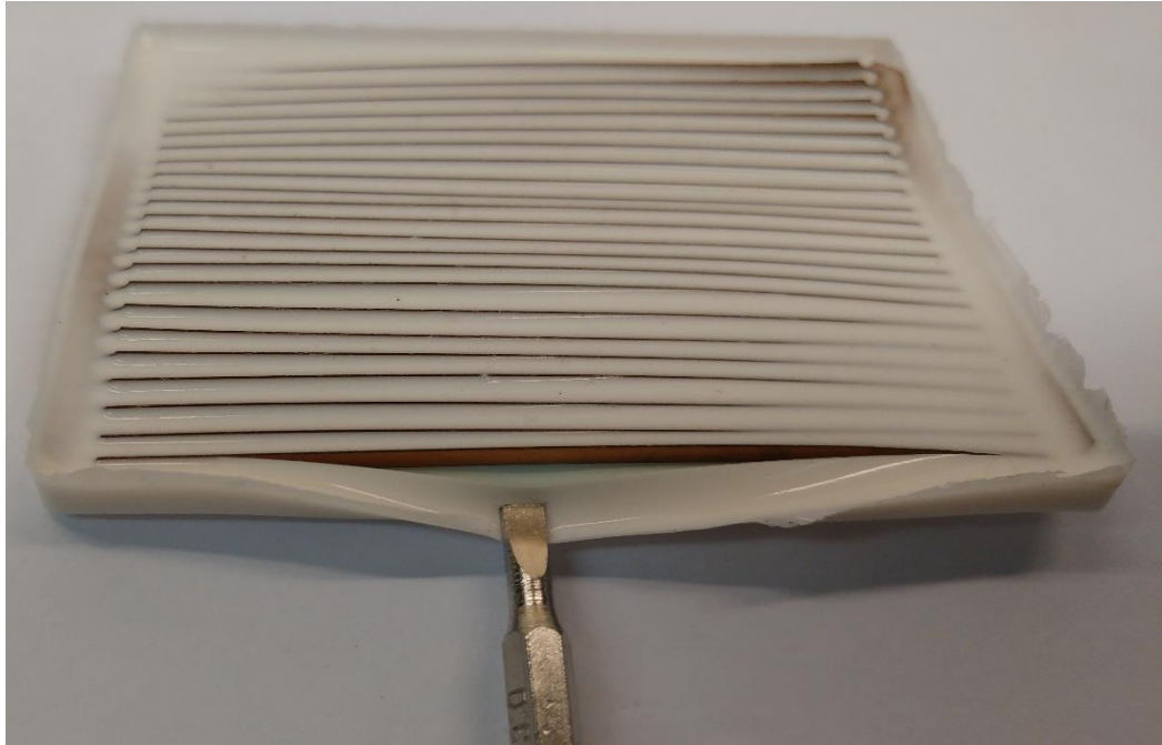
Figure 33. Detachment between copper stripes and silicone matrix (side view)
