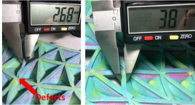
Figure 5.11 Defects on the shell thickness 2-3 mm on
