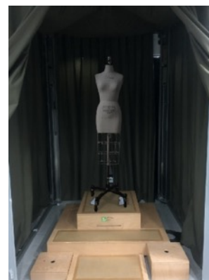
Figure 5.1 Scanning a size 10 dummy by 3D body scanner
