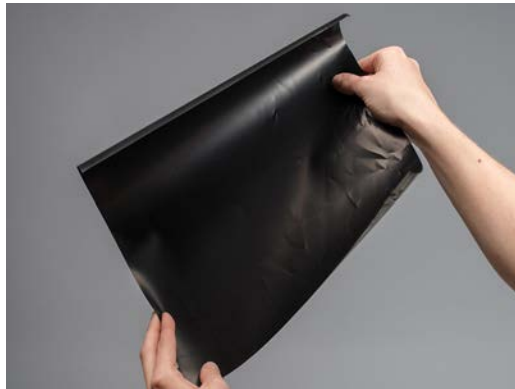
Figure 5.7 Pressure-Sensitive Conductive Sheet
