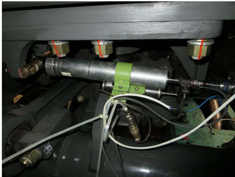
Figure 3.20 Laterally-deployed type-C MR damper in secondary suspension of tested EMU train vehicle
