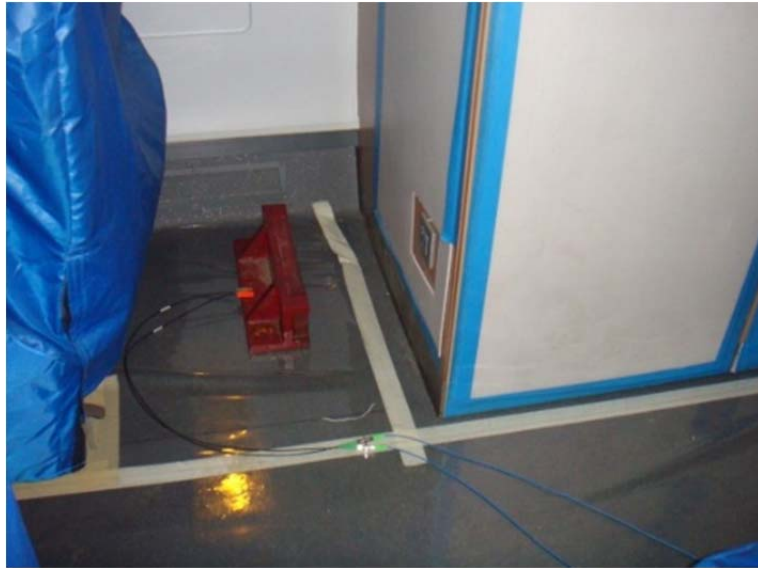
(a) Accelerometer at the floor level in car body
