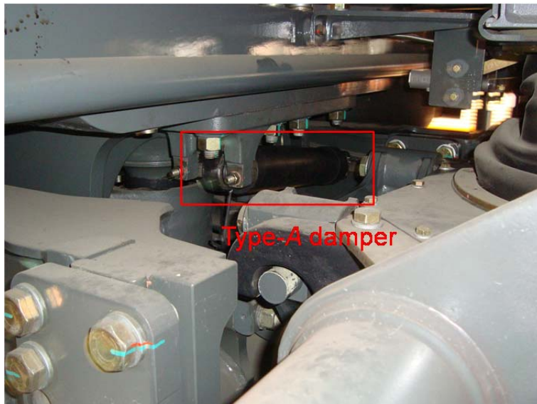
Figure 3.13 Laterally-deployed type-A MR damper in secondary suspension of tested EMU train vehicle
