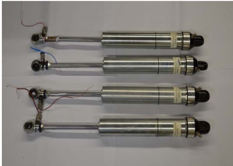
Figure 4.1 Four prototypes of new MR damper exclusive for CRH3 EMU
