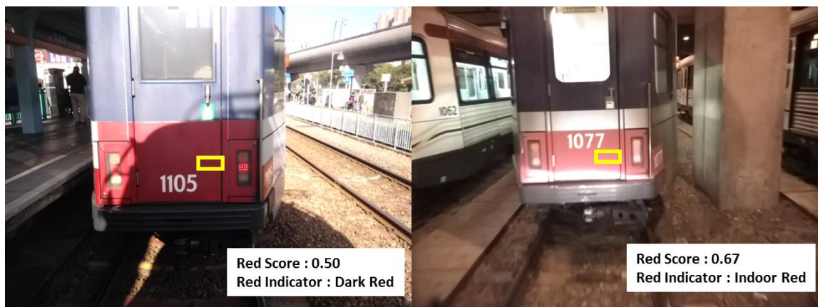
Figure 47 Example of red indicators in different conditions
