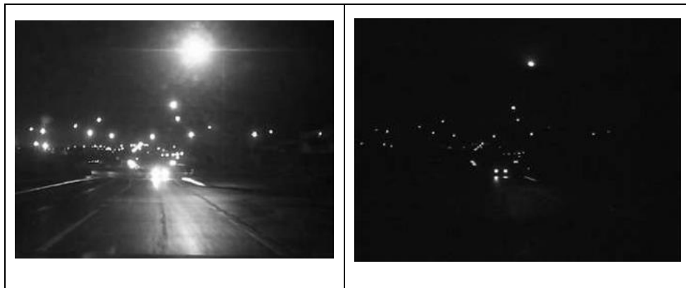
Figure 2-4. Normal exposure image (left) and low exposure image (right). Source: O'malley et al. (2011).
