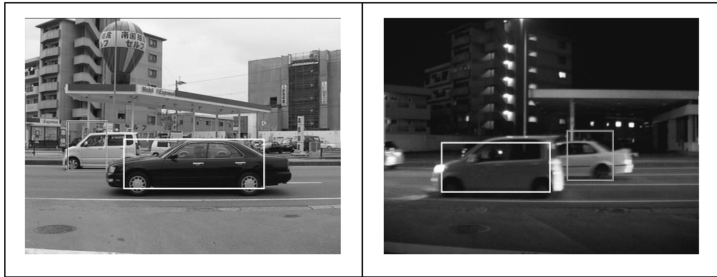
Figure 2-6. Vehicle detection using the same algorithm at daytime (left) and nighttime (right).
