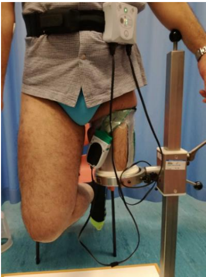
Figure 4. 8 the pressure sensor validation of the CRS socket while the patient full body weight added
