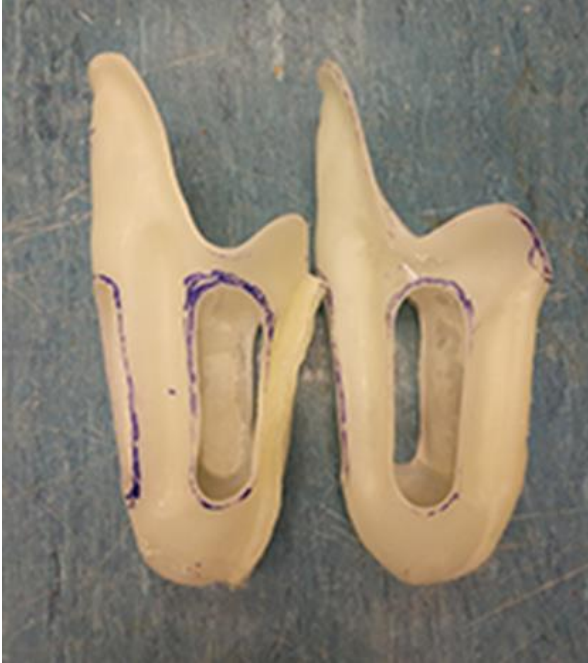
Figure 3. 6 The CRS socket. left, 10mm compression; right 15mm compression
