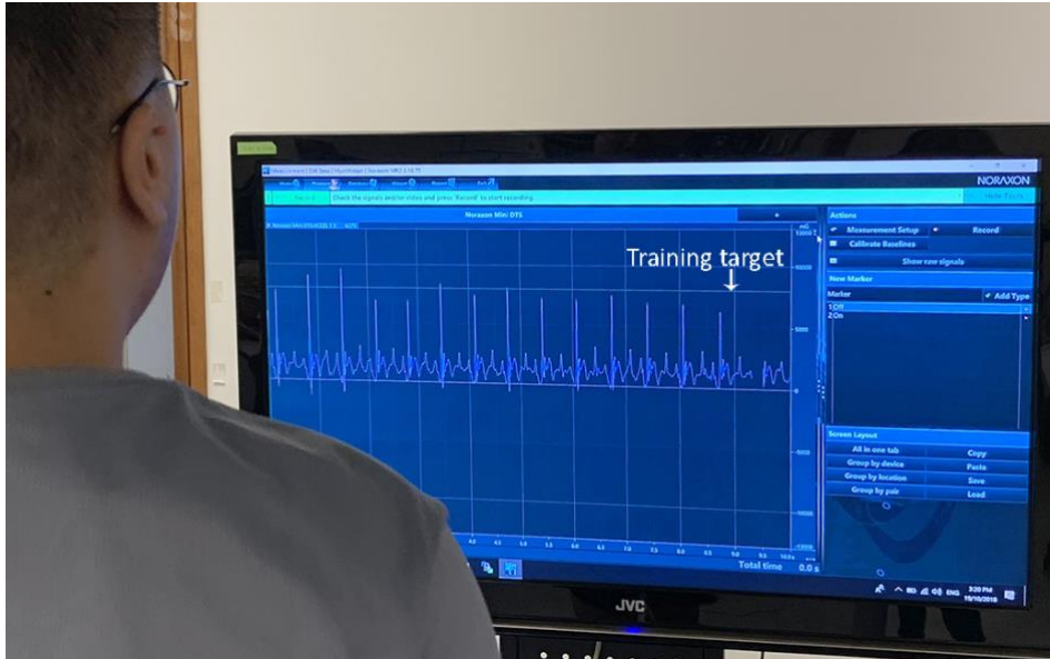
Figure 5.1 Example of real-time tibial acceleration provided to the runners as a biofeedback during gait retraining
