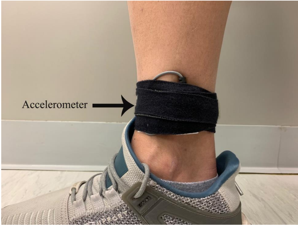
Figure 3.2 Placement of the accelerometer on the distal tibia
