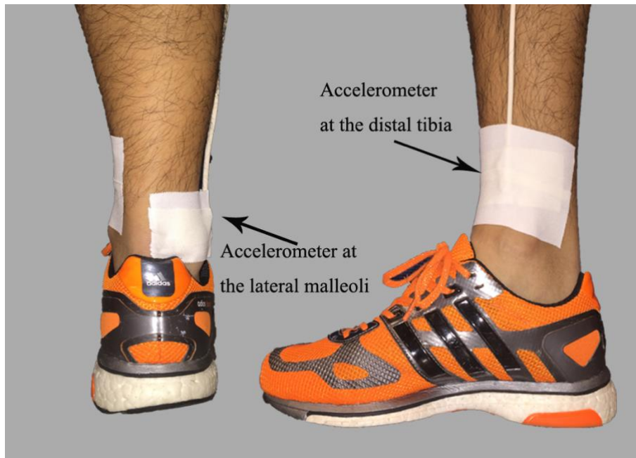
Figure 4.1 Accelerometers taped to the subject's lateral malleoli and the anteromedial aspect distal tibia
