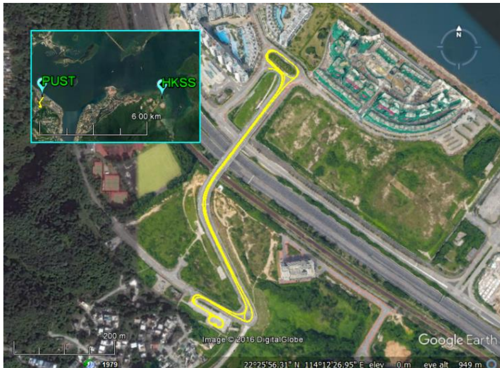
Figure 4-2 Driving trajectories in Shatin area of Hong Kong (denoted as PUST) on June 11, 2015, 08:00:00–08:33:59 (GPS time). The data is processed with HKSS as base station, about 7 km from PUST
