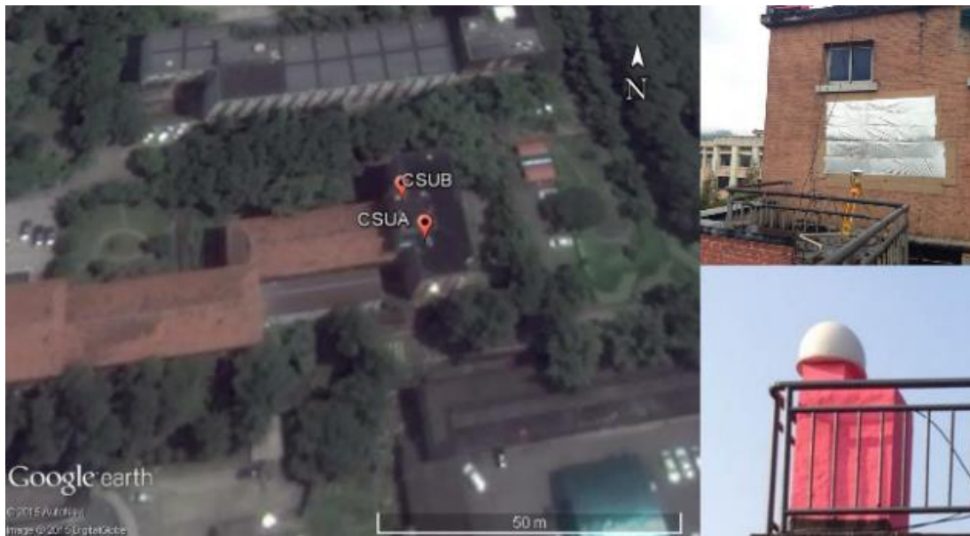
Figure 3-4 Observation sites at CSUA (upper right diagram) and CSUB (lower right diagram); Tinfoil paper was placed on the north wall near site CSUA to enhance the signal reflection
