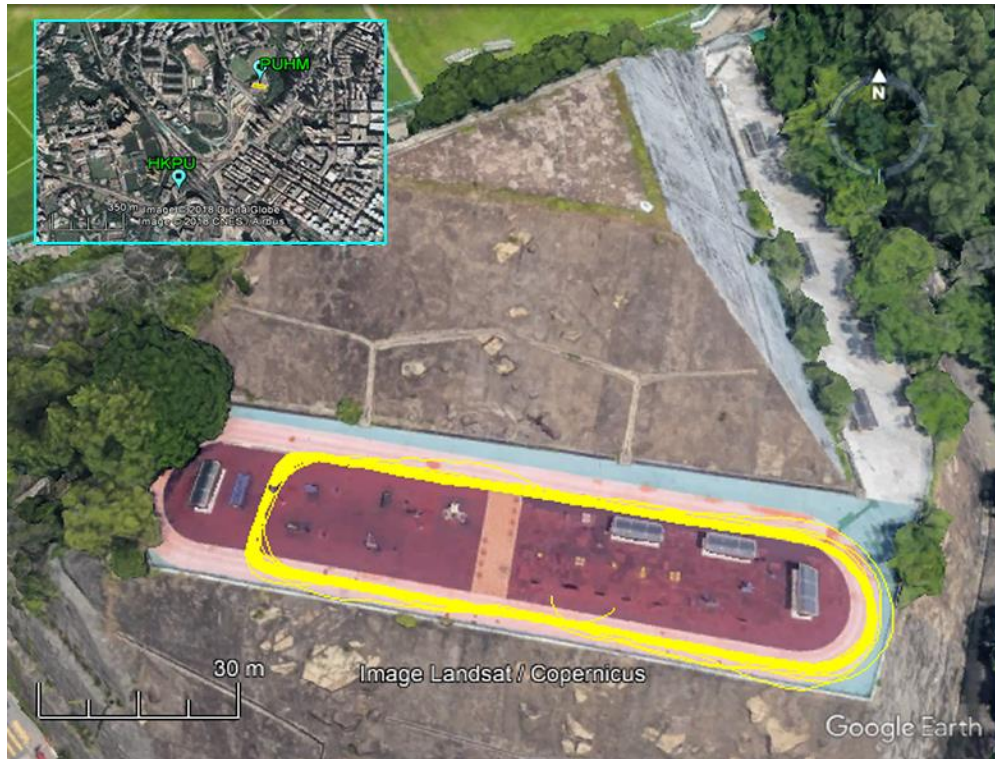
Figure 4-3 Running trajectories near a high slope in Homantin area of Hong Kong (denoted as PUHM) on July 4, 2018, 12:50:00–14:13:00 (GPS time). The data is processed with HKPU as base station, which is about 0.7 km from PUHM
