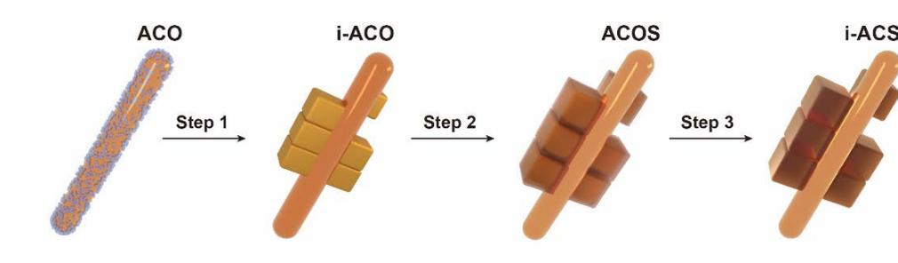
**Scheme 6.1** Schematic synthetic procedure of Au-Cu<sub>2</sub>O and Au-copper sulfide hetero-nanostructures.
