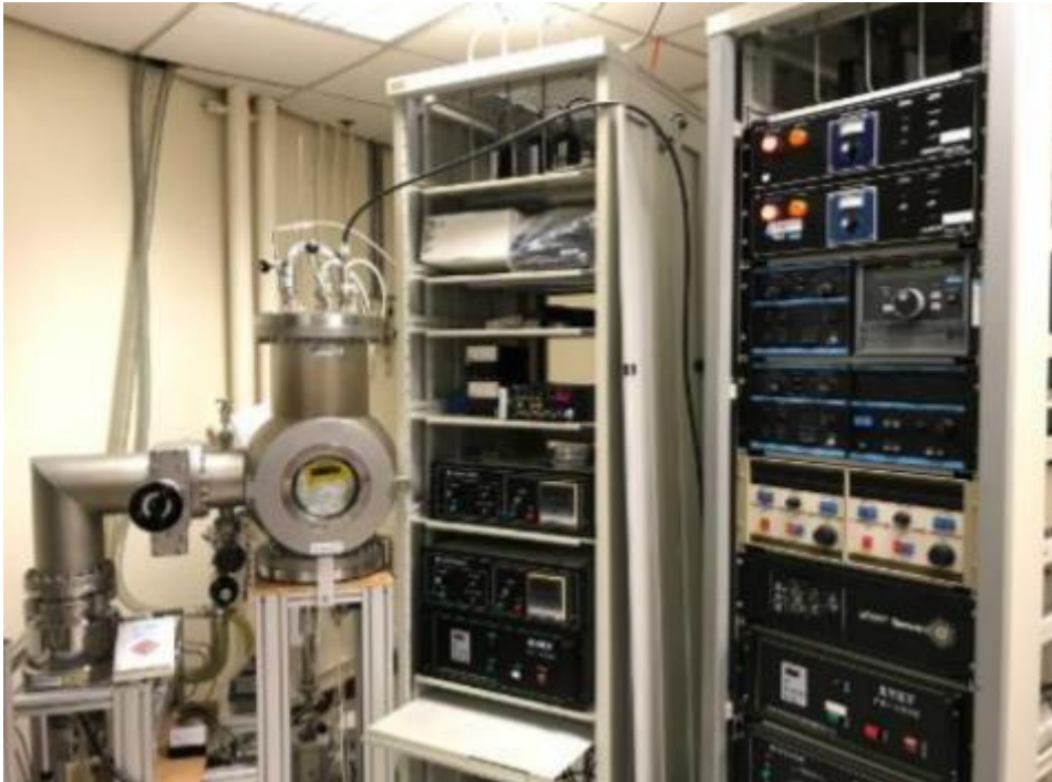
Figure 2-11 Experimental setup of a D.C. magnetron sputtering system.
