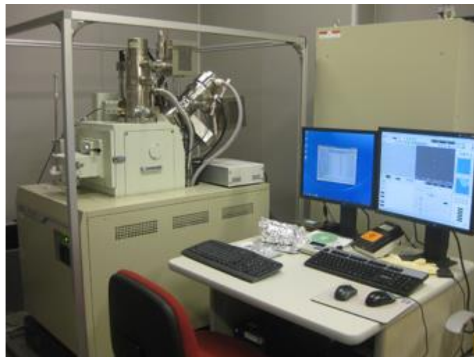
Figure 2-13 JEOL JIB-4501 scanning electron microscope equipped with the module of nano-pattern generation system.
