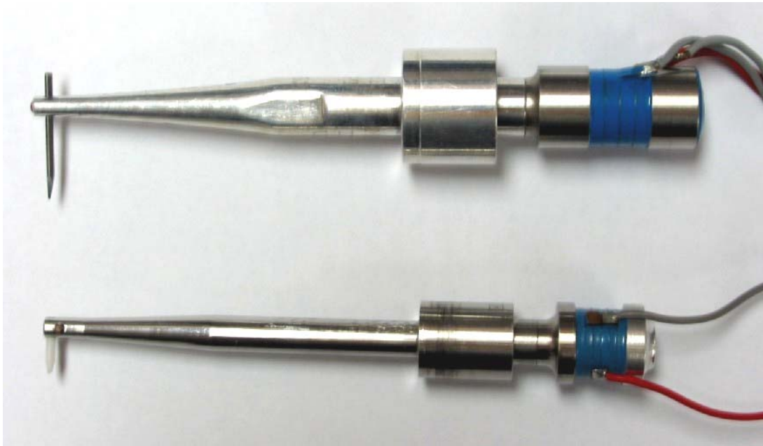
Fig. 1.12 Commercial ultrasonic wire bonding transducers.
