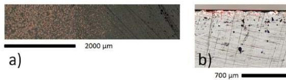
Figure 1.2 (a) A photo of the surface of  $\text{Cu}_2\text{S}$  pellet fabricated using the SPS method, (b) a photo of the cross-section of the  $\text{Cu}_2\text{S}$  sample (G. Dennler et al., 2014).
