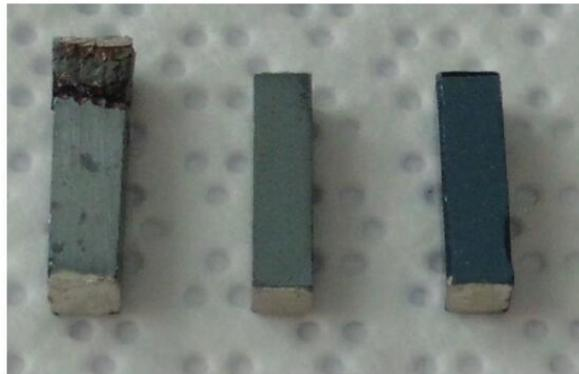
Figure 1.3 From left to right:  $\text{Cu}_2\text{Se}$  sample after current stress of  $24 \text{ A cm}^{-2}$  for 24 h,  $\text{Cu}_{1.8}\text{S}$  and  $\text{CuS}$  samples after current stress of  $48 \text{ A cm}^{-2}$  for 72 h, respectively (G. Dennler et al., 2014).
