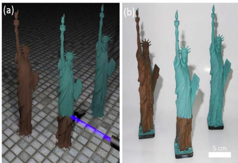
Figure 5.8. 3D printed Statue of Liberty with coating of malachite. (a) schematic image; (b) real product.
