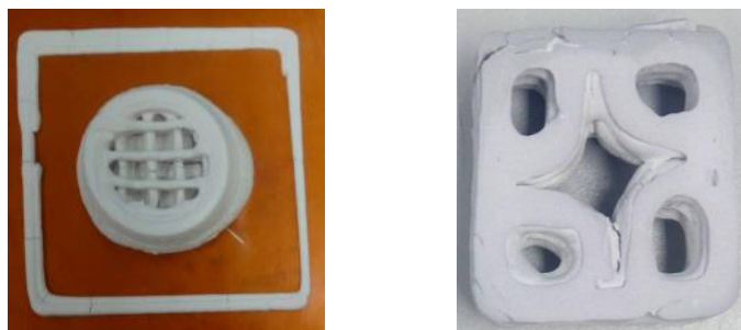
Figure 6.8 3D printed structures of AlN ceramics.
