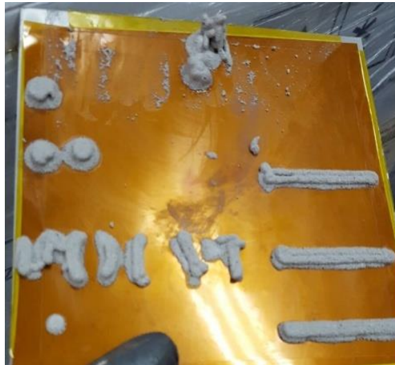
Figure 6.13 3D printing using recycled AlN for the fourth time.
