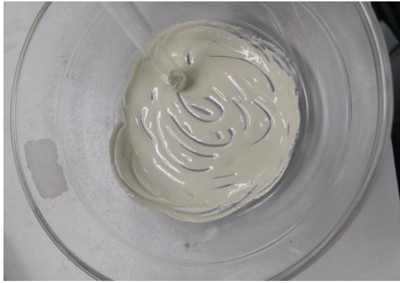
Figure 4.2 AlN/ovalbumin gelcasting slurry.
