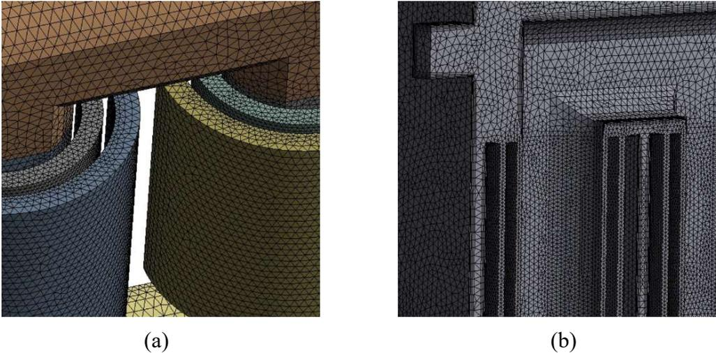
Fig. 5.2. Mesh of (a)core, windings, and (b) oil.
