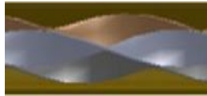
Triple twisted tape [57]
