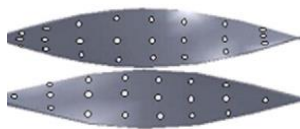
Perforated double counter twisted tape [58]
