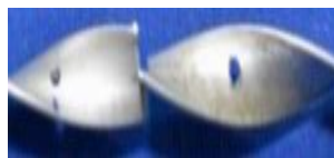
Perforated twisted tapes with alternate axis [102]
