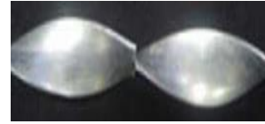
Alternate clockwise and counter clockwise twisted tapes [51]
