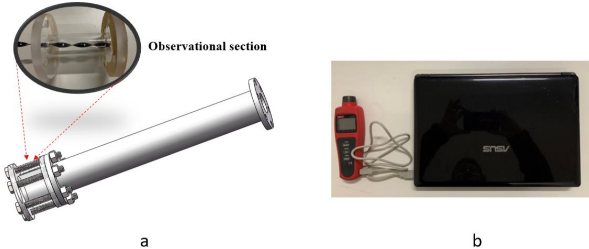
Figure 5.2 (a) The circular tube designed with observational section; (b) Rotational speed measurement: Digital tachometer RPM meter with contactless mode
