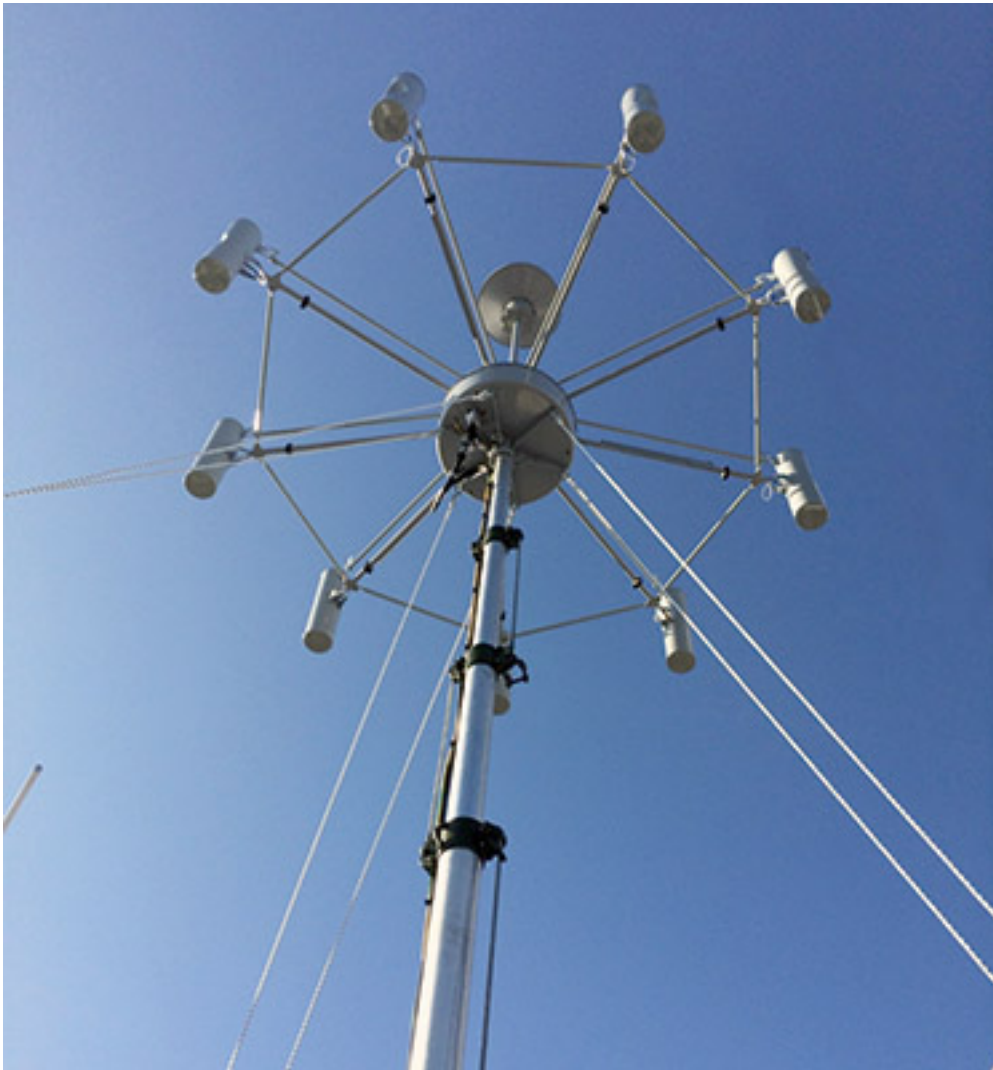
Figure 1.1: Circular array of antenna system, company name ARTIKUL-S direction finder. This is design by IRCOS company [1].
