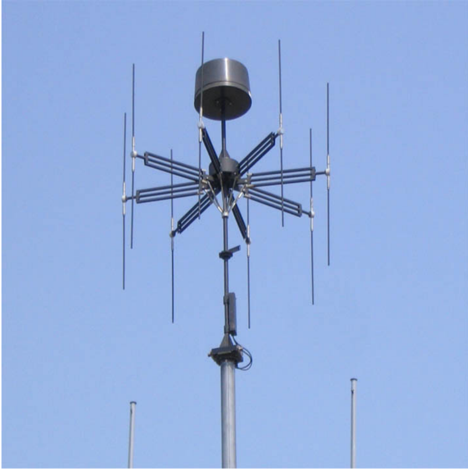
Figure 1.2: Circular array round-the-clock radio navigation, security and unauthorized sources of radiation detection in the Republic of Armenia [2].
