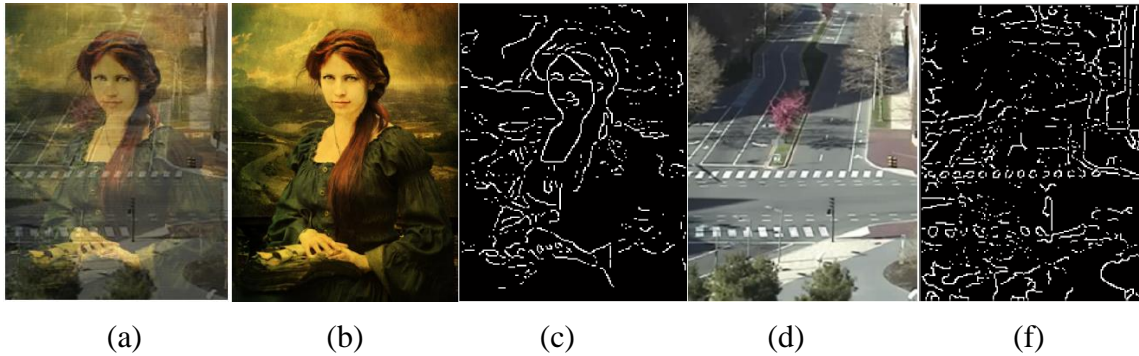
Fig. 2.2. One example to illustrate the gradient independence property [9]. (a) is obtained by superimposing (d) on (b). (c) and (e) are the strong gradients of (b) and (d) respectively.
