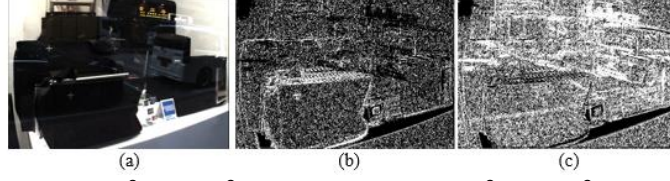
Fig. 3.5(i). An example of E_B^0 and E_R^0 . We can see that E_B^0 and E_R^0 can roughly separate the background and reflection gradient components.
