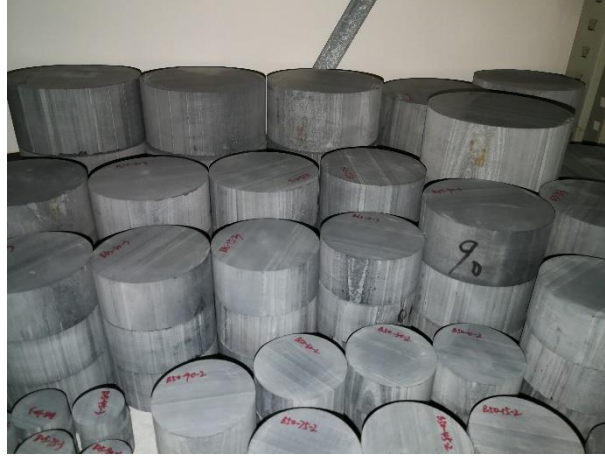
Figure 4.4 Preparation of disc slate samples of various diameters
