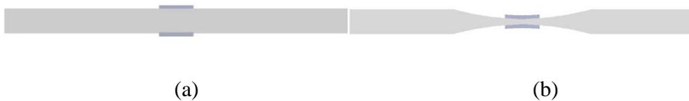
Figure 4.2 Reference plate and ABH plate coated with the same amount of damping layers. Coating area  $x_{d1} \sim x_{d2}=0.25\sim 0.31\text{ m}$ ,  $y_{d1} \sim y_{d2}=0\sim 0.56\text{ m}$  and thickness  $h_d=2h_0$ :
