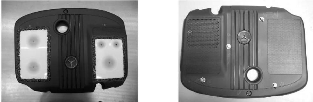
Figure 1.9 ABH engine cover (top view) and locations of accelerometers on reference engine cover [92].
