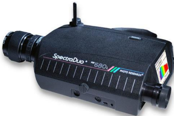
Figure 2-9 A spectroradiometer for color temperature and CIE coordinates measurement.
