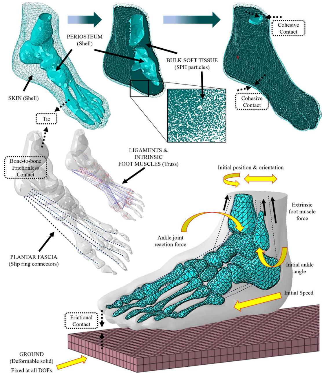
**Figure 32. Overview of finite element foot model setup and boundary conditions.**
