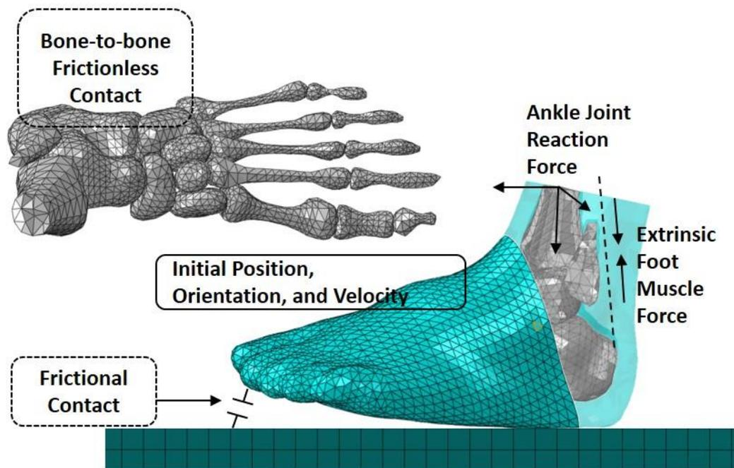
**Figure 27. Boundary/loading conditions for the running simulations.**
