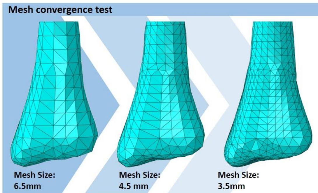
*Figure 28. Mesh size refinement for the finite element models. From left to right, the general mesh size of the distal tibia is reduced from 6.5 mm to 3.5 mm.*
