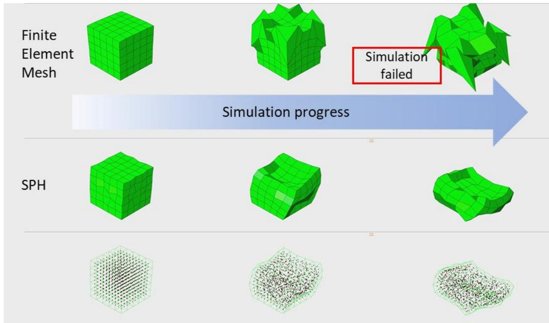
*Figure 26. Modeling cube using either finite element mesh or SPH particles and the simulation results.*
