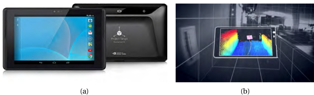
FIGURE 2.11: Google's Project Tango tablet and demo simulation. (a) Project Tango Developer Toolkit. (b) RGB-D image simulation. © Google Copyright 2015
