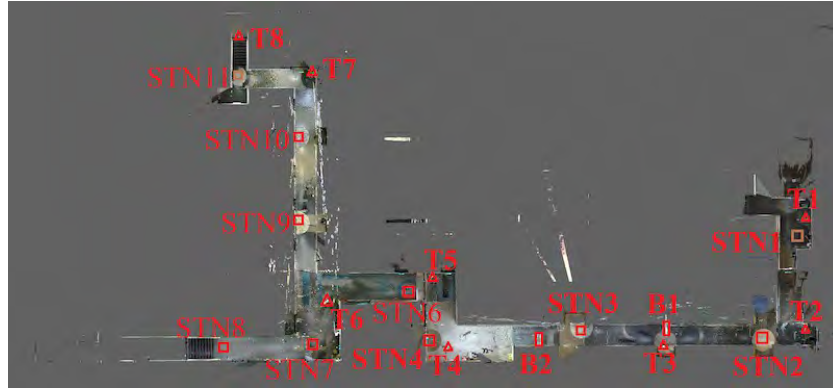
FIGURE 4.26: The distribution of the scan stations, which are rectangles labeled "STN1" to "STN11", targets, which are triangles labeled "T1" to "T9", and vertical reference boards used as extra references labeled "B1" and "B2".
