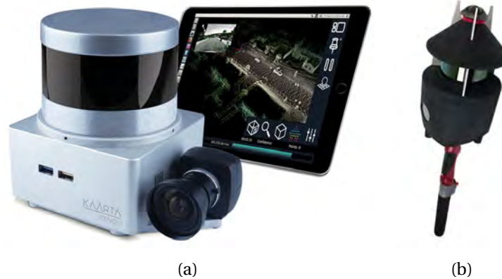
FIGURE 2.22: Portable integrated mobile mapping solutions by startup companies. (a) Kaarta Stencil2, integrating an Intel NUC, a Velodyne VLP-16 scanner, a fisheye camera, and an IMU inside, with a tablet for control and data visualization © Kaarta Copyright 2019. (b) Paracosm PX-80 which is similar to Kaarta Stencil2 but with different installation and processing workflow © Occipital Copyright 2019.
