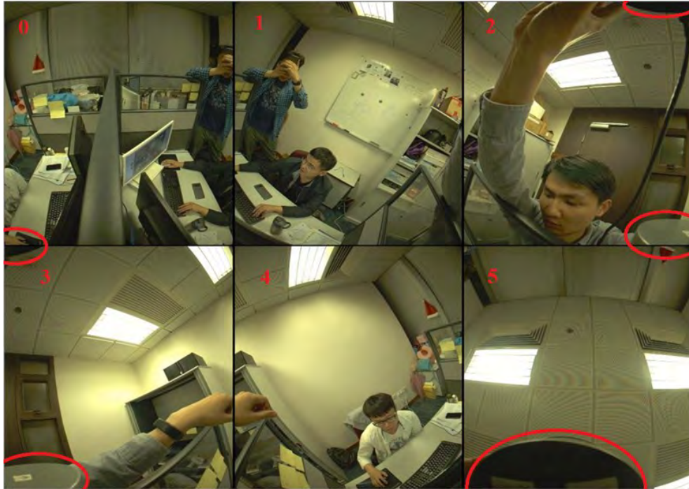
FIGURE 4.5: The example of neighboring sensors blocking part of the panoramic FOV of the camera. For the six cameras numbered from 0-5, the top right and bottom right corners of camera 2, the top left and bottom left corners of camera 3, and the lower part of camera 5, which are all marked with red circles, are blocked by the two laser scanners beside the camera lens.
