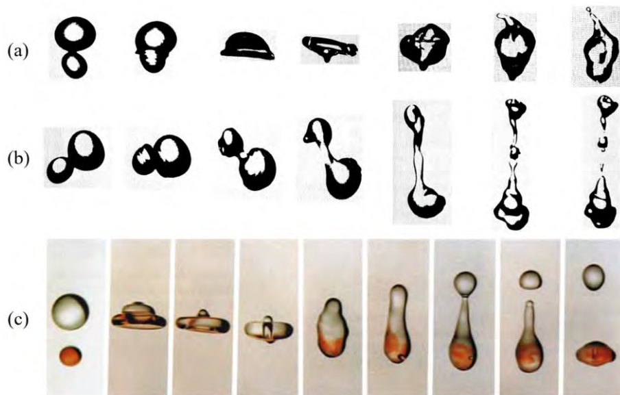
Figure 2.4 Experimental images of collision between two droplets of unequal sizes: water droplets of \Delta = 1.41 , We \approx 20 [10] at (a) B = 0.0 and (b) B = 0.9 , and (c) water droplets of \Delta = 2.0 , We = 56 and B = 0.0 [14].
