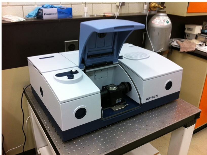
Figure 3.3 Bruker attenuated total reflection FTIR spectrometer
