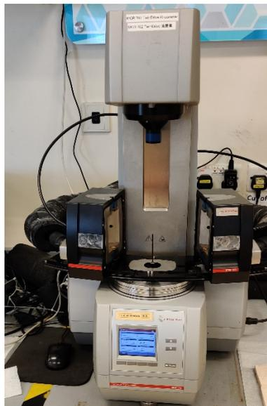
Figure 3.6 Dynamic shear rheometer (DSR)
