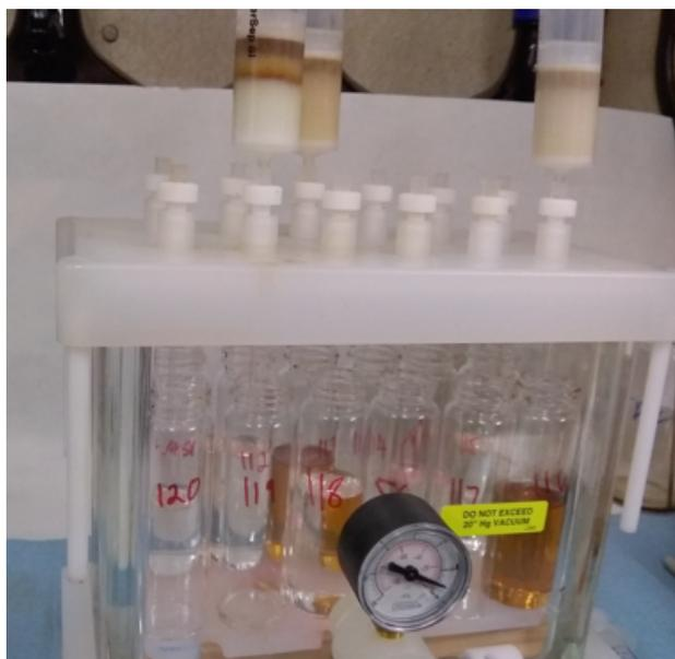
Figure 5.5 Elution of aromatics through SPE cartridges [119]
