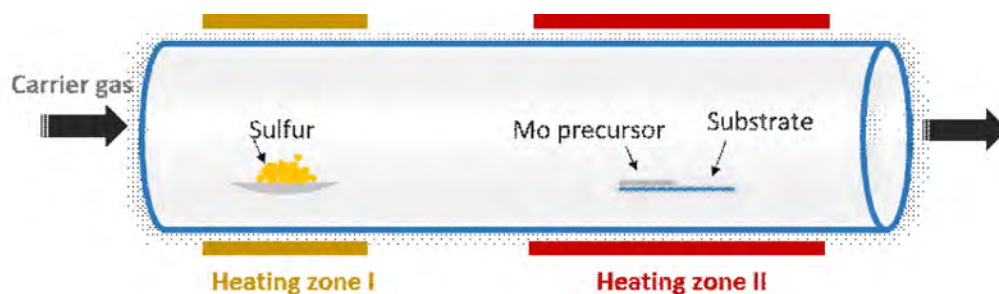
Figure 3.11 Setup for the sulfurization of pre-deposited metal film.
