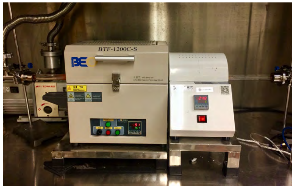
Figure 2.3 Schematic diagram of the homemade CVD system.
