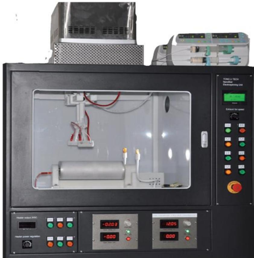
**Fig. A3.1.**Electrospinning apparatus used for spinning PVDF fibrous filters in this study.
