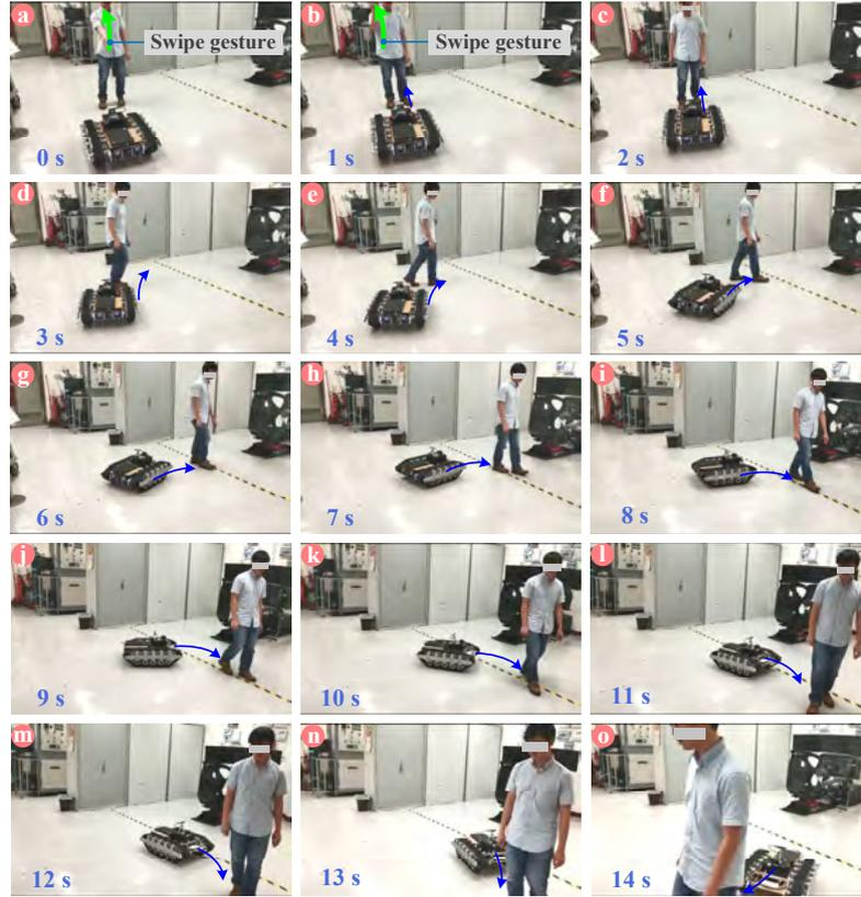
**Fig. 6.11:** Snapshot sequence: human-robot following control in a curved path. (a-b) Controller is activated by the swipe-up hand gesture. (c-o) Following process in a curved path.
