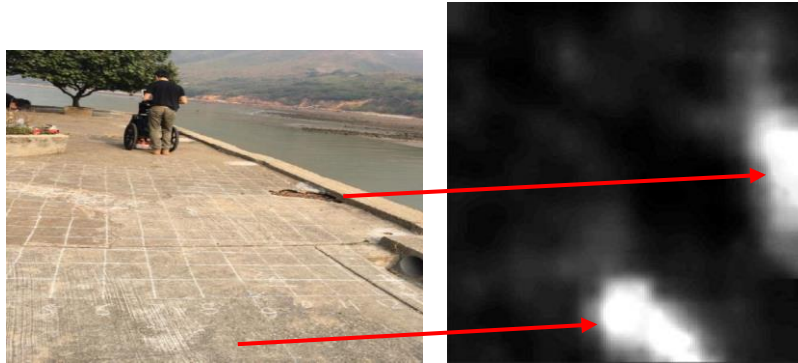
Figure 5-12 Tai O site and its C-scan at 40cm deep
