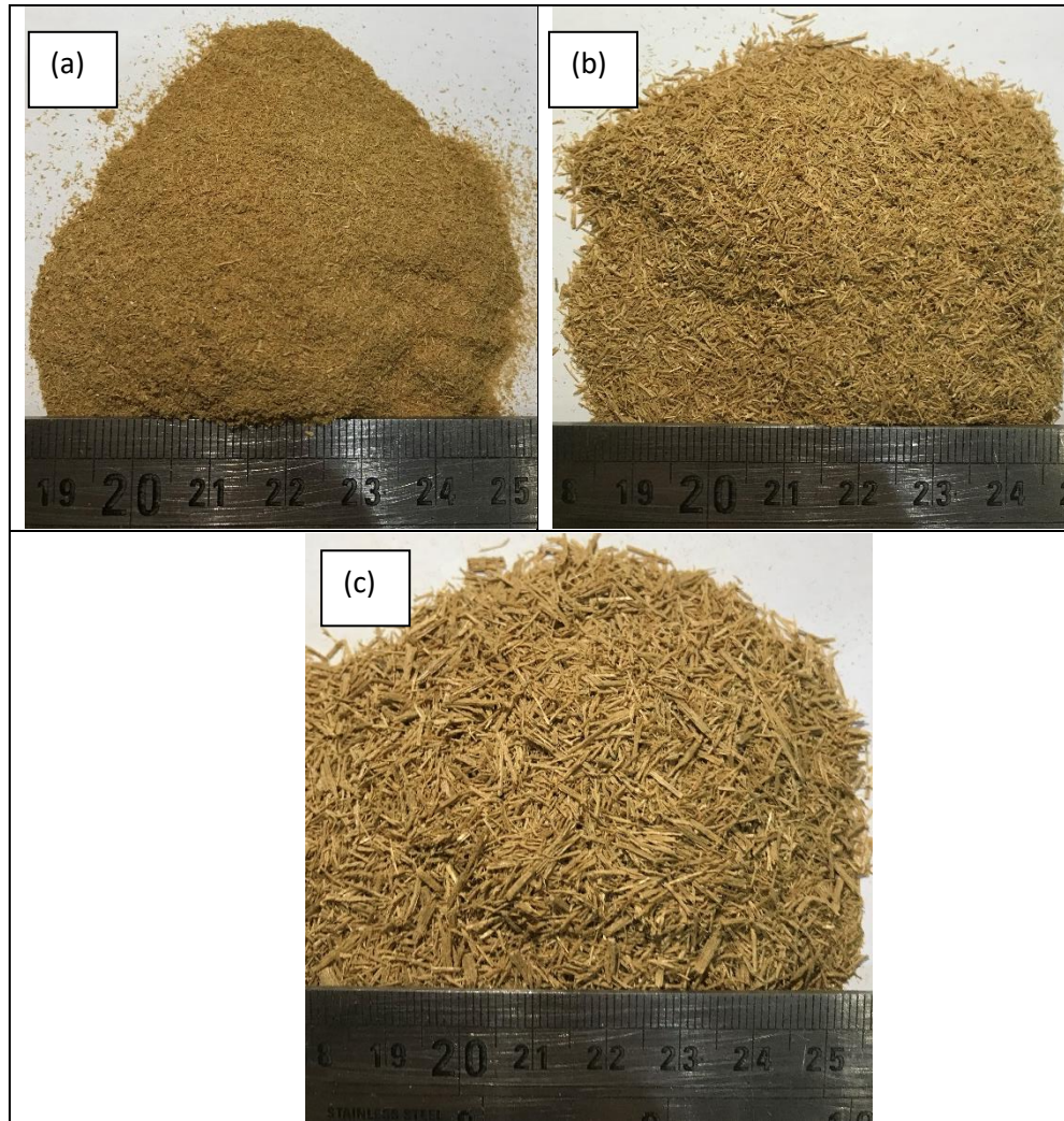
Figure 7-1 Wood fibres with different lengths (a) Fine (b) Medium (c) Coarse
