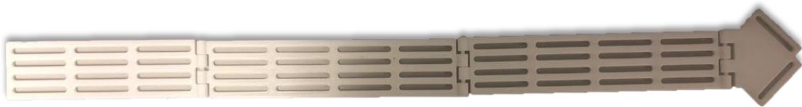
Figure 5-14 Schematic of artificial back bone with hinged joint
