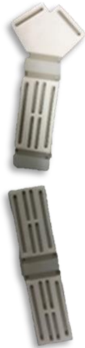
Figure 5-13 Broken off resin joint
