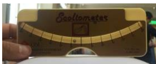
Figure 3-2 OSI scoliometer used for ATR measurement
