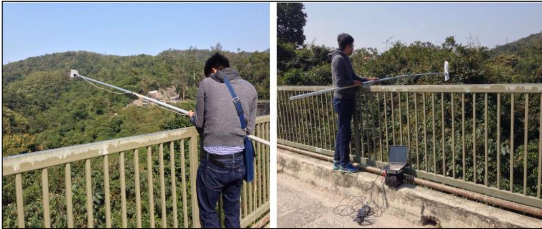
Figure 4-16: Acquiring vegetation spectra using two different spectral radiometers
