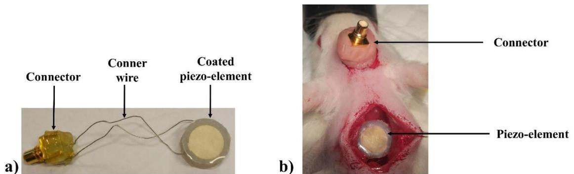
**Fig 16: Ultrasound stimulation probe; a)** A piezoelectric element was coated with silicone and connected to a connector via Teflon coated wires; **b)** The probe was placed on the cervical region after dorsal column crush and the connector was mounted on the head using dental cement.
