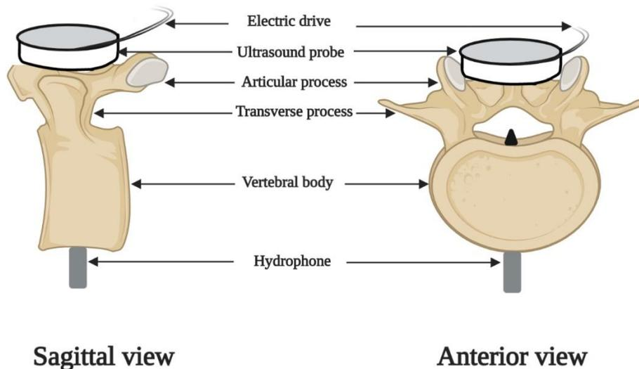
**Fig. 19: *Ex-vivo* setup to measure the ultrasound intensity inside the vertebral canal** (10 mm diameter probe used to generate ultrasound; acoustic frequency 1 MHz, 20% duty cycle, PRF 1 kHz).
