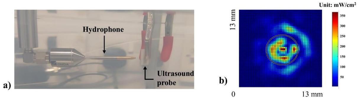
**Fig. 18: Ultrasound intensity measurement in a water tank.** a) In a water tank, a hydrophone was placed front side of the tank. b) Scanning result from one ultrasound probe ( $I_{SATA}$  value =  $67.35 \text{ mW/cm}^2$ ).
