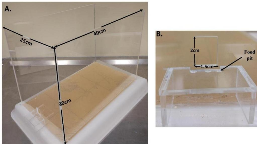
**Fig 13: Food pellet chamber;** A) Special Plexiglas chamber for reaching and grasping task; B) Small pit for food pellet. A small platform was attached outside the pit to place the
