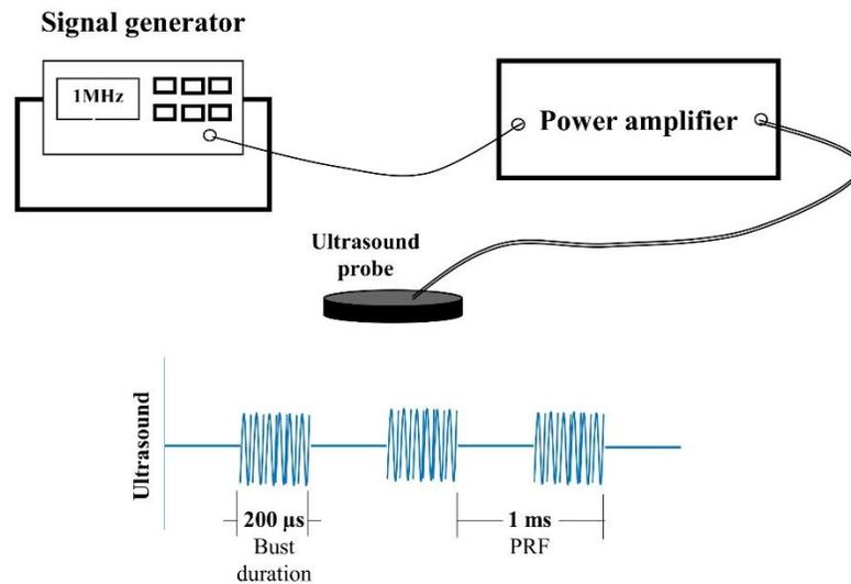
**Fig 17: Ultrasound stimulation parameter.** A custom-made ultrasound probe with an acoustic frequency of 1 MHz, 20% duty cycle and 1 ms (PRF) pulse repetition frequency were used to generate the LIPUS.
