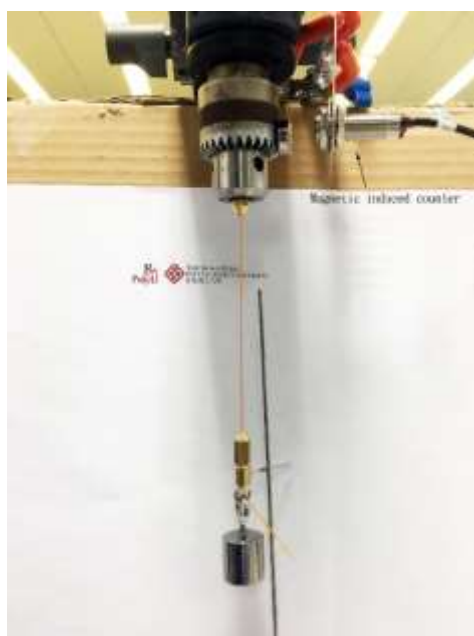
Figure 4. 1 Experimental setup for fabricating thermally powered actuator
