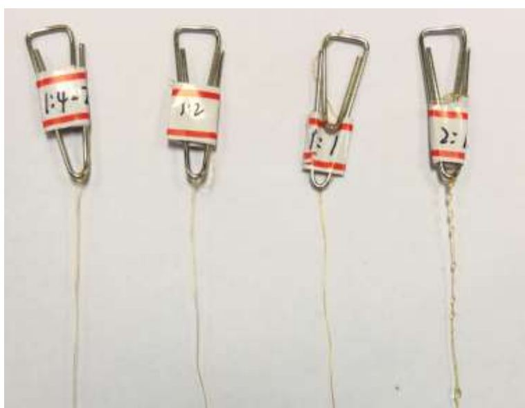
Figure 3. 6 PI/PDMS composite yarns coated by PDMS/ethyl acetate solution of different concentrations (from left to right: 1:4, 1:2, 1:1 and 2:1)
