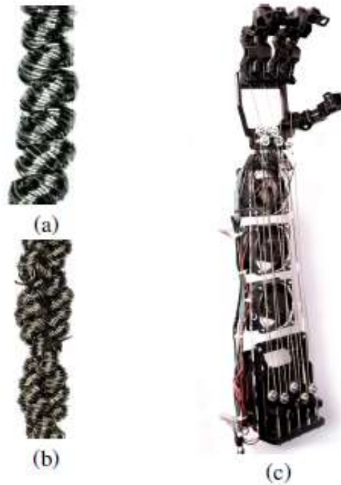
Figure 2. 20 Robotic muscles made by conductive nylon sewing thread
