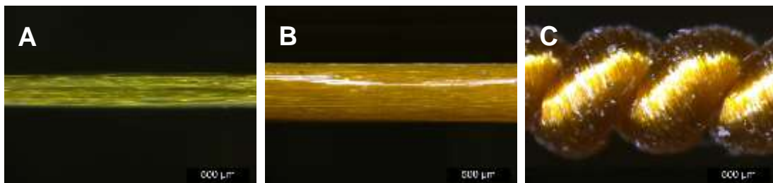
Figure 4. 5 Each state of sample for fabricating an PI/PDMS HCYA. (A) 100f PI yarn (B) 6*100f PDMS-coated PI yarn (C) 6*100f PI/PDMS HCYA
