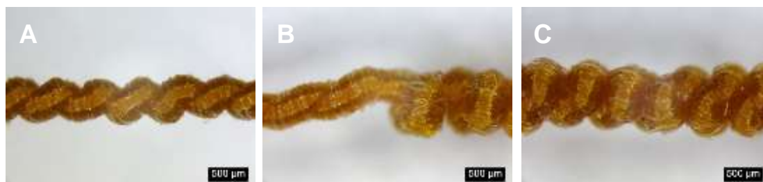
Figure 4. 6 Thermally powered HCYAs of different coil levels. (A) HCYA with single-level coil (B) HCYA with single-double-mixed-level coil (C) HCYA with double-level coil
