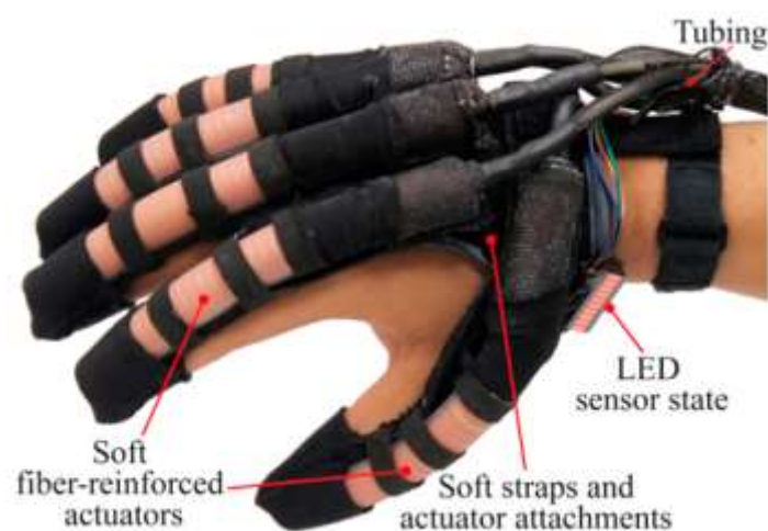
Figure 2. 3 Soft robotic glove made by hydraulic actuator for rehabilitation of handicapped hand
