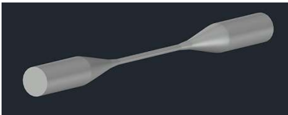
Fig. 1.6 The typical structure of a piece of fiber taper.
