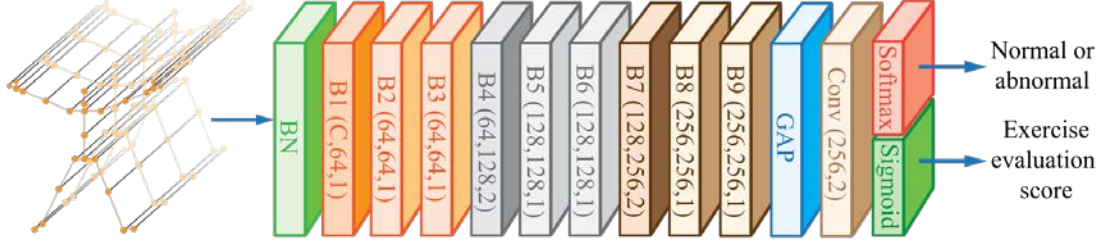
Figure 6.4 Illustration of the 2T-GCN model. There are 9 GCN blocks (B1-B9). The three numbers of each layer indicate the numbers of input and output channels, and the stride. GAP is a global average pooling layer.
