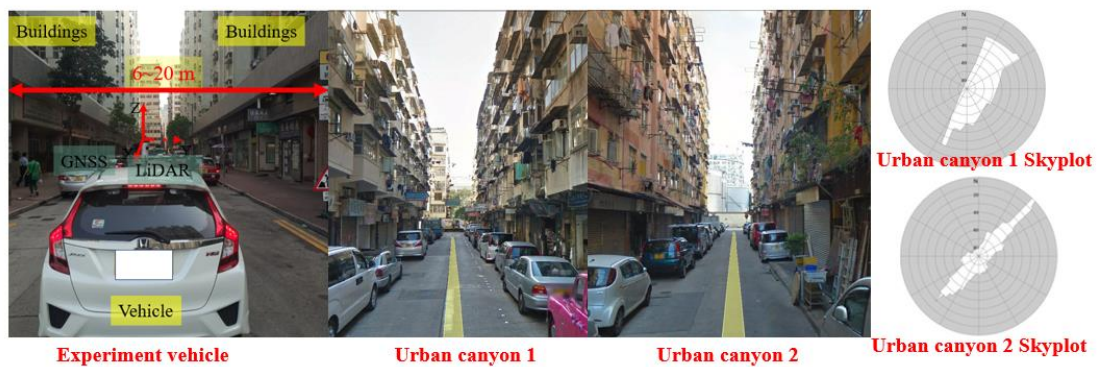
Figure 3-7. The sensors setup of the vehicle and tested environment: GNSS and LiDAR sensors are installed on the top of the vehicle shown in the left side of the figure. The two tested urban scenarios are shown in the middle of the figures. The Skyplot of the two experiments is shown on the right side of the figure.
