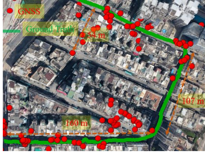
Figure 4-9. Experiment 1: Trajectory of the autonomous vehicle is indicated by the green curve. The red circles indicate the GNSS positioning result.
