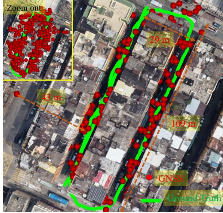
Figure 4-13. Experiment 2: Trajectory of the vehicle is indicated by the green curve. The red circles indicate the object detection aided GNSS positioning results.
