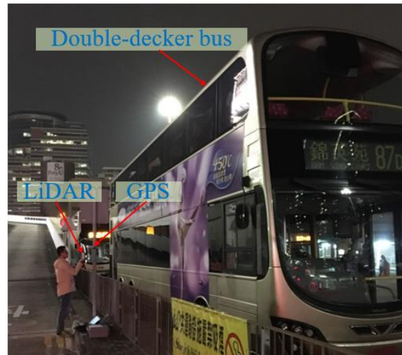
Figure 2-5 An environment that the data were collected at a bus stop. Satellites can be blocked by the double-decker bus.
