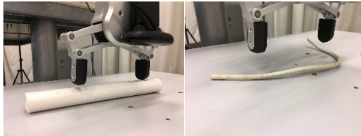
Figure 20. Failure occurred when only one gripping method is set
