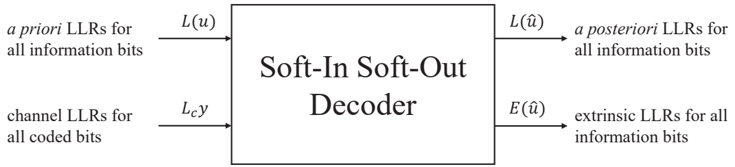
Figure 2.3: Illustration of a soft-in soft-out decoder.
