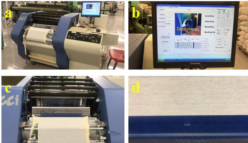
**Fig 5.1** Photographs showing (a) the weaving system. (b) the control software. (c) weaving process. (d) the obtained fabric during weaving.
