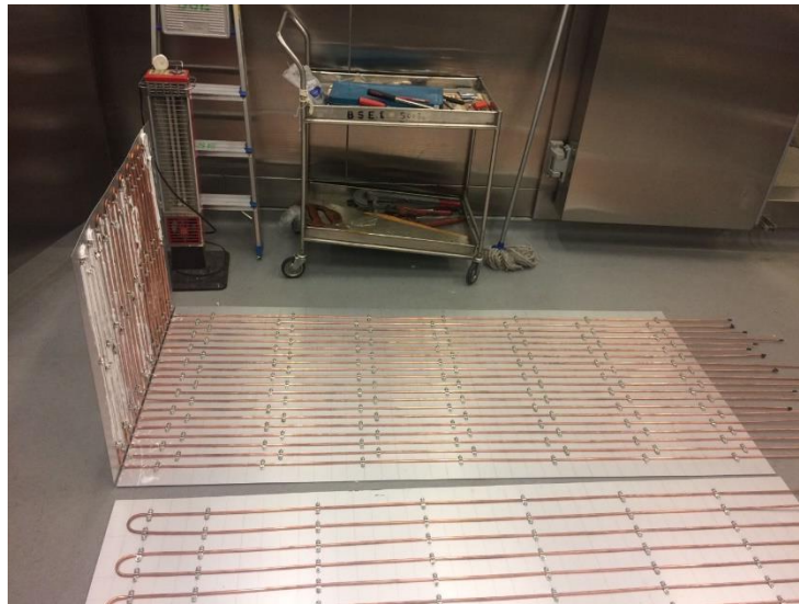
(b) V-Section of the bed-based heating terminal
