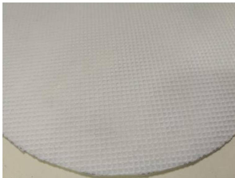
Fig 4.8 Surface photo of a PTFE HEPA medium
